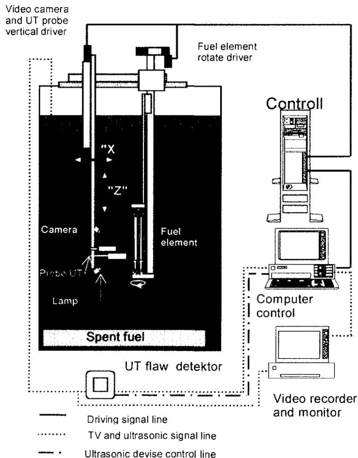
of computer controlled servomotor; with 1/deg accuracy for rotation movement and 0,1 mm accuracy for Z axis movement,
