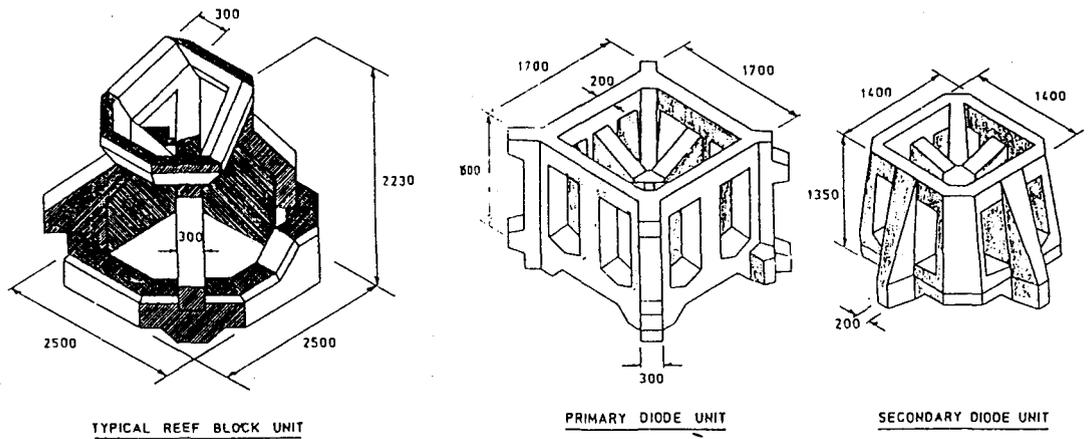
FIGURE 6: Isometric Detail of Armour Units
