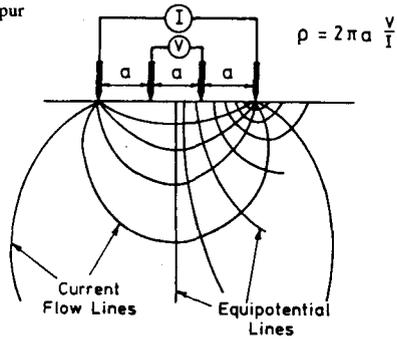
FIGURE 4: Resistivity Meter
