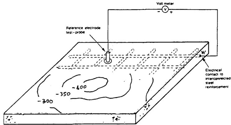
FIGURE 1: Half cell and Potential Plot
