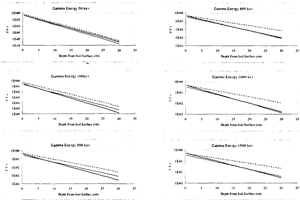
FIGURE 1. Ratio of Radiation Flux at 100 cm from Soil Surface, to the Flux of a Layer of Radionuclide at Different Burial Depths, for Different Photon Energies. Dotted Lines by Simple Model, Solid Lines by Simulations and Thin Lines by Modified Mathematical Model.
