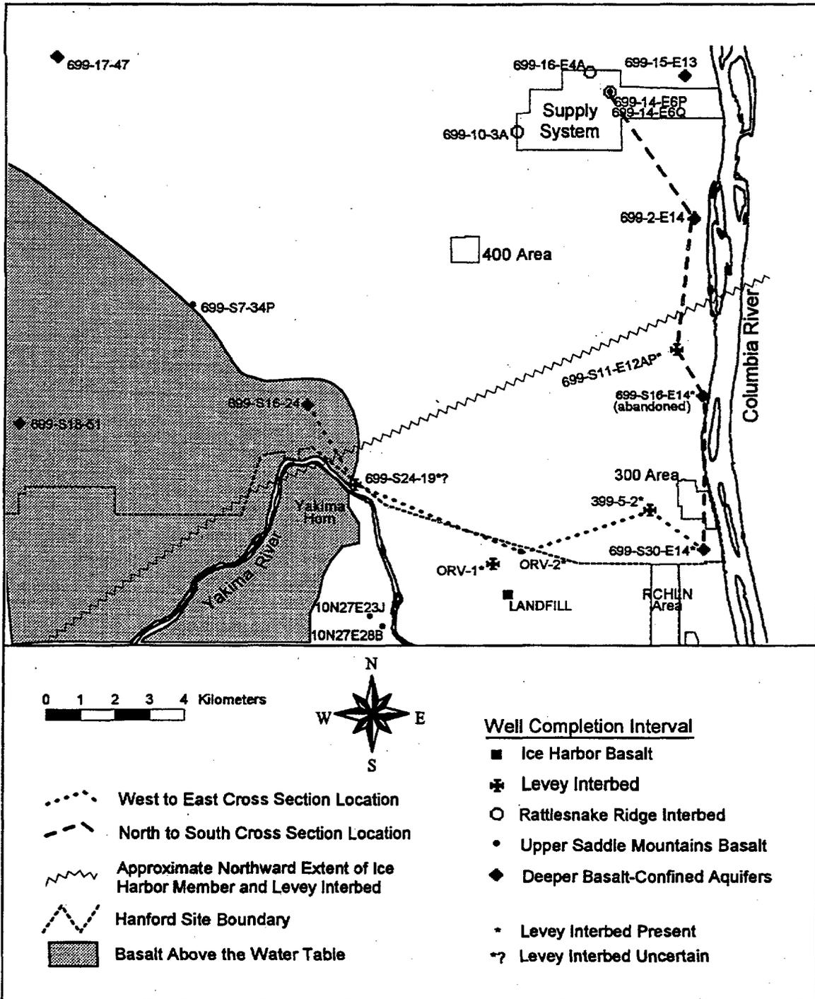
**Figure 1.** Basalt-Confined Aquifer Wells in the Southern Part of the Hanford Site and Cross Section Locations
