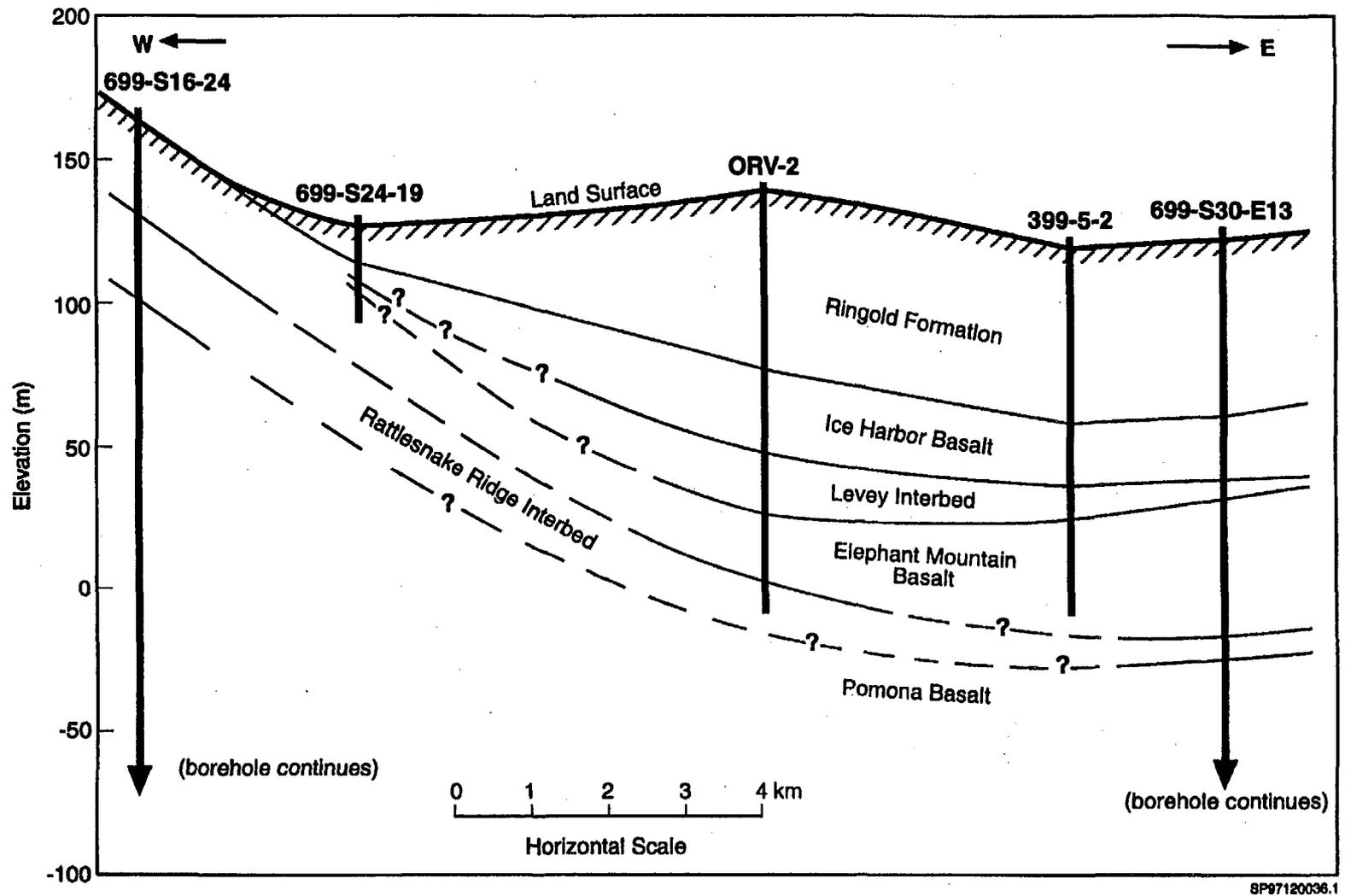
Figure 2. West to East Cross Section Near the Southern Site Boundary (see Figure 1 for location)
