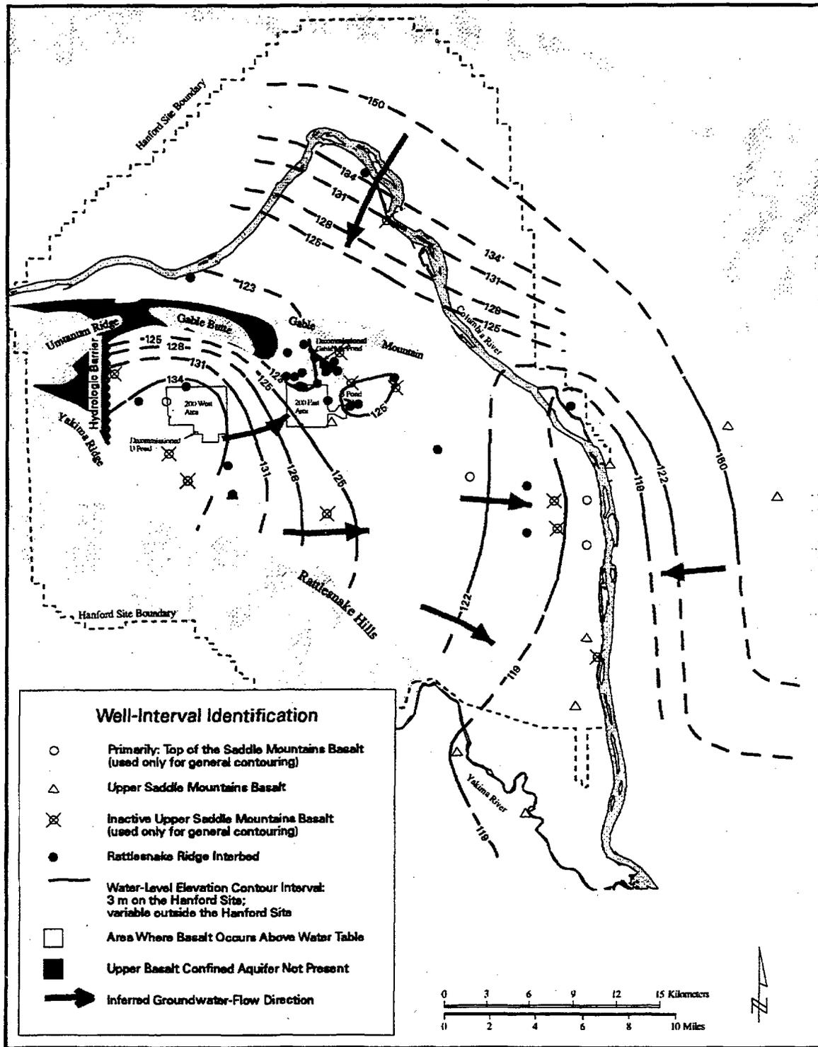
**Figure 5.** Potentiometric Map of the Upper Basalt-Confined Aquifer System – March 1993
