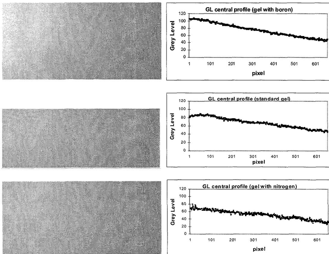
Fig. 5. Transmittance images and Grey Level profiles of gels with the various compositions.
