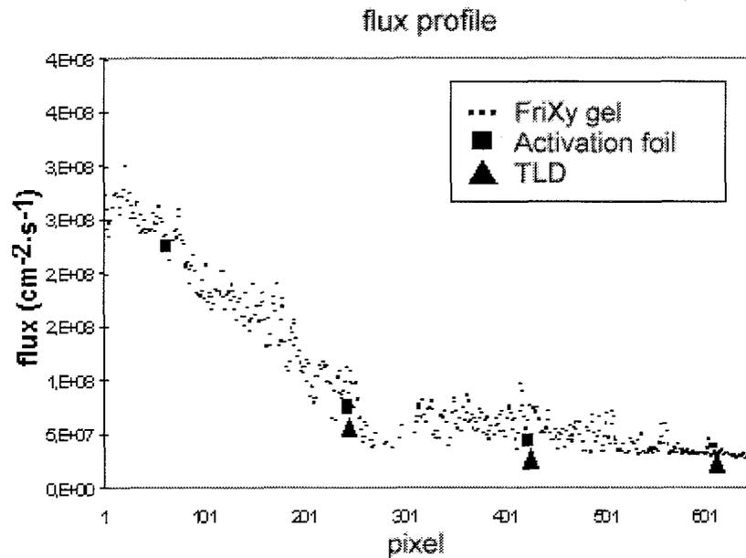
FIG.7. Inter-comparison of flux profile obtained with FriXy-gel and fluxes measured with activation foils and with TLDs.
