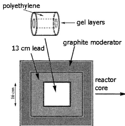
FIG. 3a. Moderator and irradiation set up.
