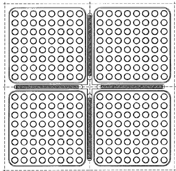
Fig. 1: Cruciform Absorber Blades in a BWR Lattice.
