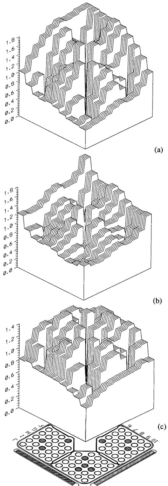
**Fig. 4:** Distribution of Average Integral Parameters for the Controlled SVEA-96+ Assembly: (a)  $F_{tot}$ , (b)  $C_B$ , and (c) the reaction rate ratio  $F_{tot}/C_B$ .
