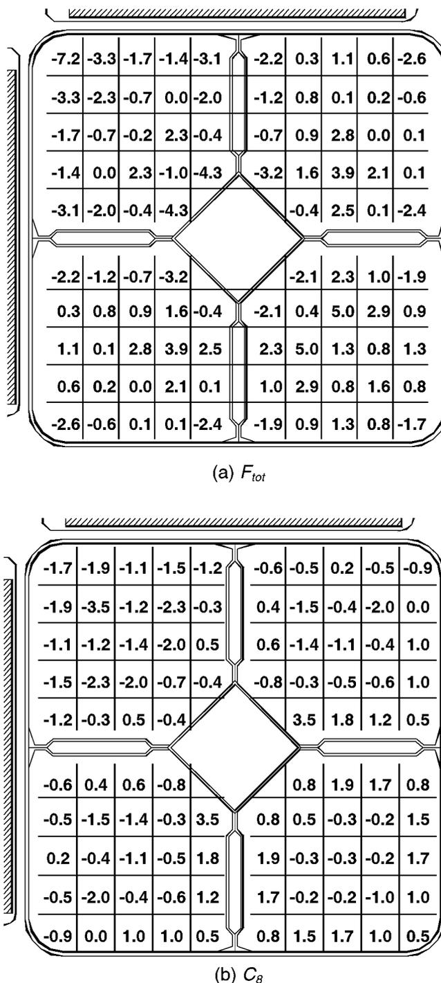
Fig. 5: CASMO/BOXER-1 Results (in %) for (a) Total Fission Rate, and (b)  $^{238}\text{U}$ -Capture Rate.
