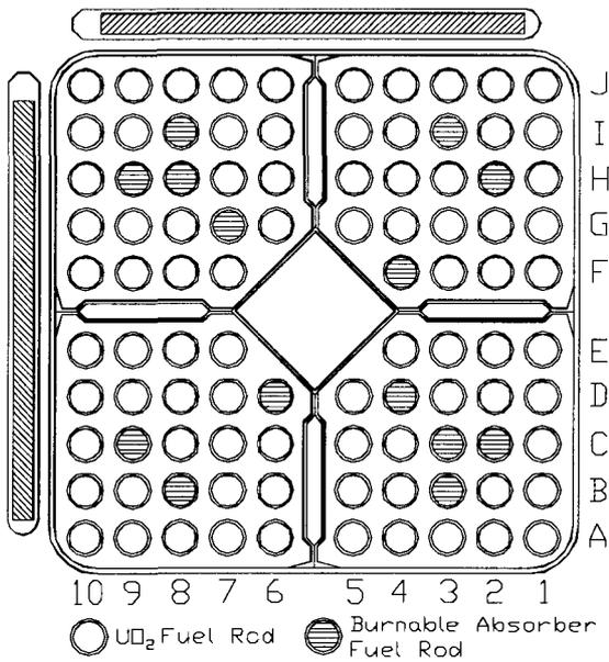
**Fig. 3:** Westinghouse SVEA-96+ Assembly Geometry.
