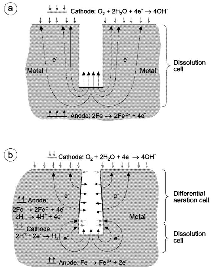
Fig. 1: Description of stress corrosion cracking: (a) by the Coupled Environment Fracture Model and (b) by the PLEDGE model.
