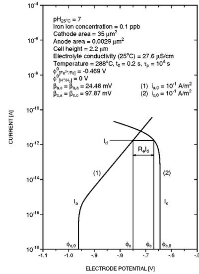
**Fig. 4:** Determination of the anodic and cathodic potentials and the dissolution current  $I_d$ .
