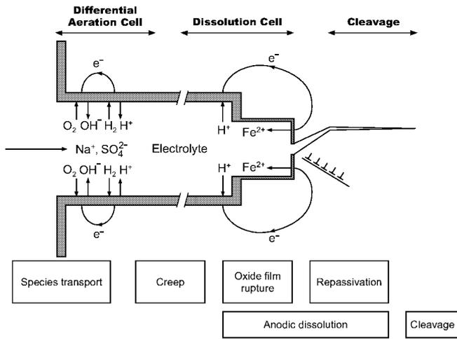
**Fig. 2:** Phenomena assumed to be involved in stress corrosion cracking of low-alloy steels in high temperature water.
