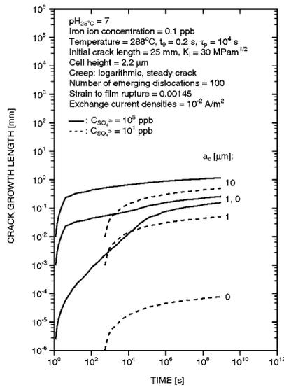
Fig. 9: Calculated crack growth length versus time.
