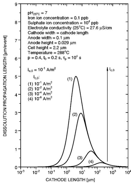
**Fig. 7:** Dissolution propagation length versus cathode length.
