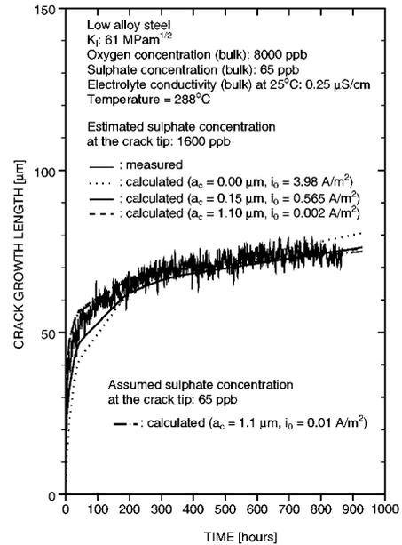
Fig. 10: Qualitative comparison of the crack growth length calculated from the model with that measured [1,2].
