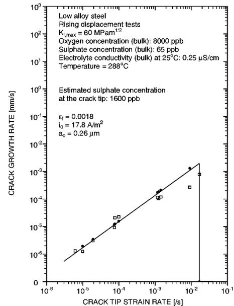
Fig. 11: Crack growth rate versus crack tip strain rate obtained by Rising Displacement Tests ( $\square$ , [1]), and by the present model ( $\bullet$ , [2]).
