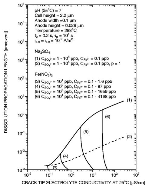
**Fig. 8:** Dissolution propagation length versus conductivity for two electrolytes of different compositions.
