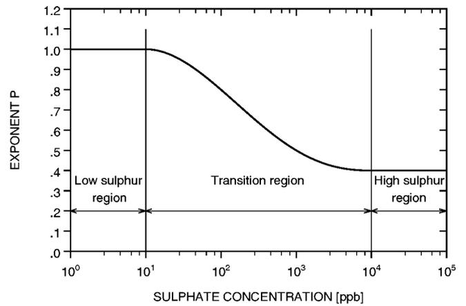
**Fig. 6:** Value of  $p$  versus sulphate concentration.
