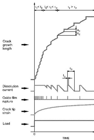
**Fig. 5:** Load versus time and resulting strain at the crack tip, oxide film rupture events, dissolution current, and crack growth length.
