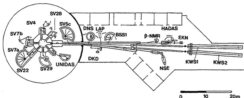
Figure 1: Layout of the DIDO reactor and ELLA with instrument positions.
