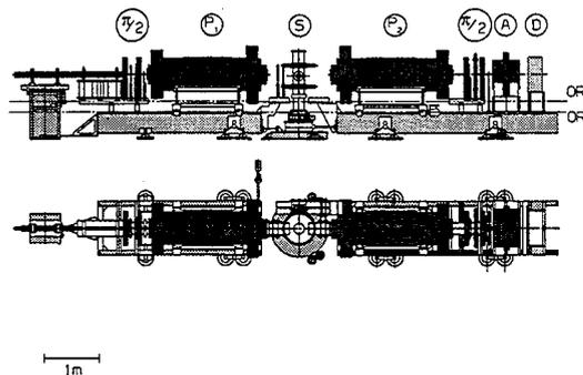
Figure 5: Mechanical layout for the NSE spectrometer. Most conspicuous the two symmetric main precession coils with compensating loops at both ends.
