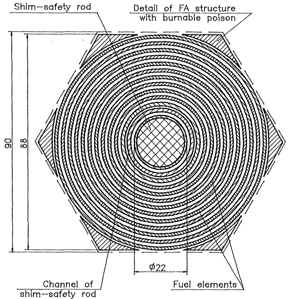
Figure 2. Cross-section of the FA with tubular-type fuel elements.
