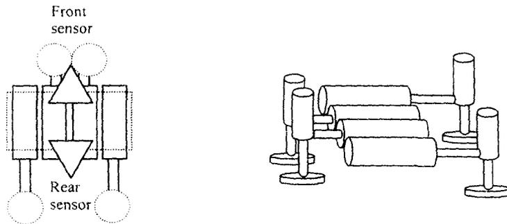
Figure 5. The location of photoelectric sensors and the overall structure
