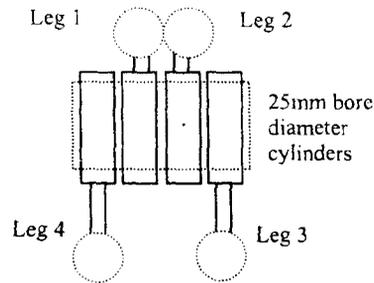
Figure 1. The large cylinders are arranged parallel where two are facing up and another two down
