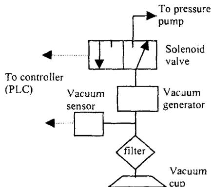
Figure 3. The vacuum system devices and pressure sensor (control signal)
