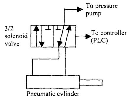
Figure 4. The cylinder system with the control signal
