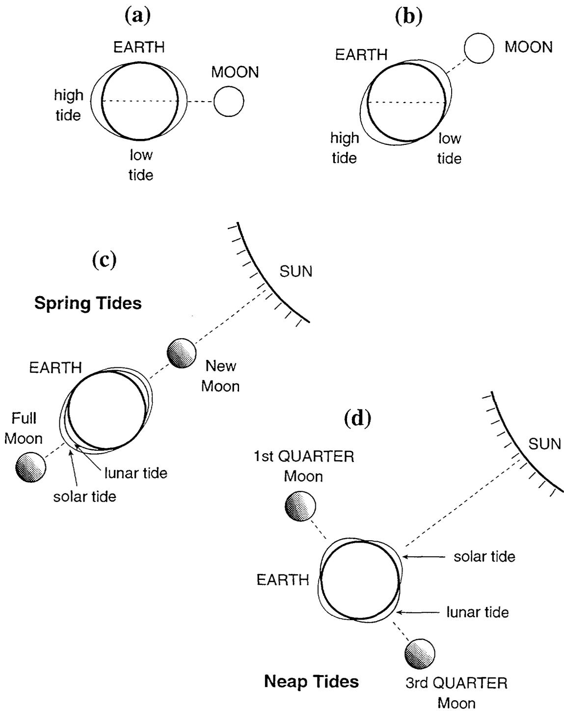
FIG. 12. Schematic representation showing how tides are created.
