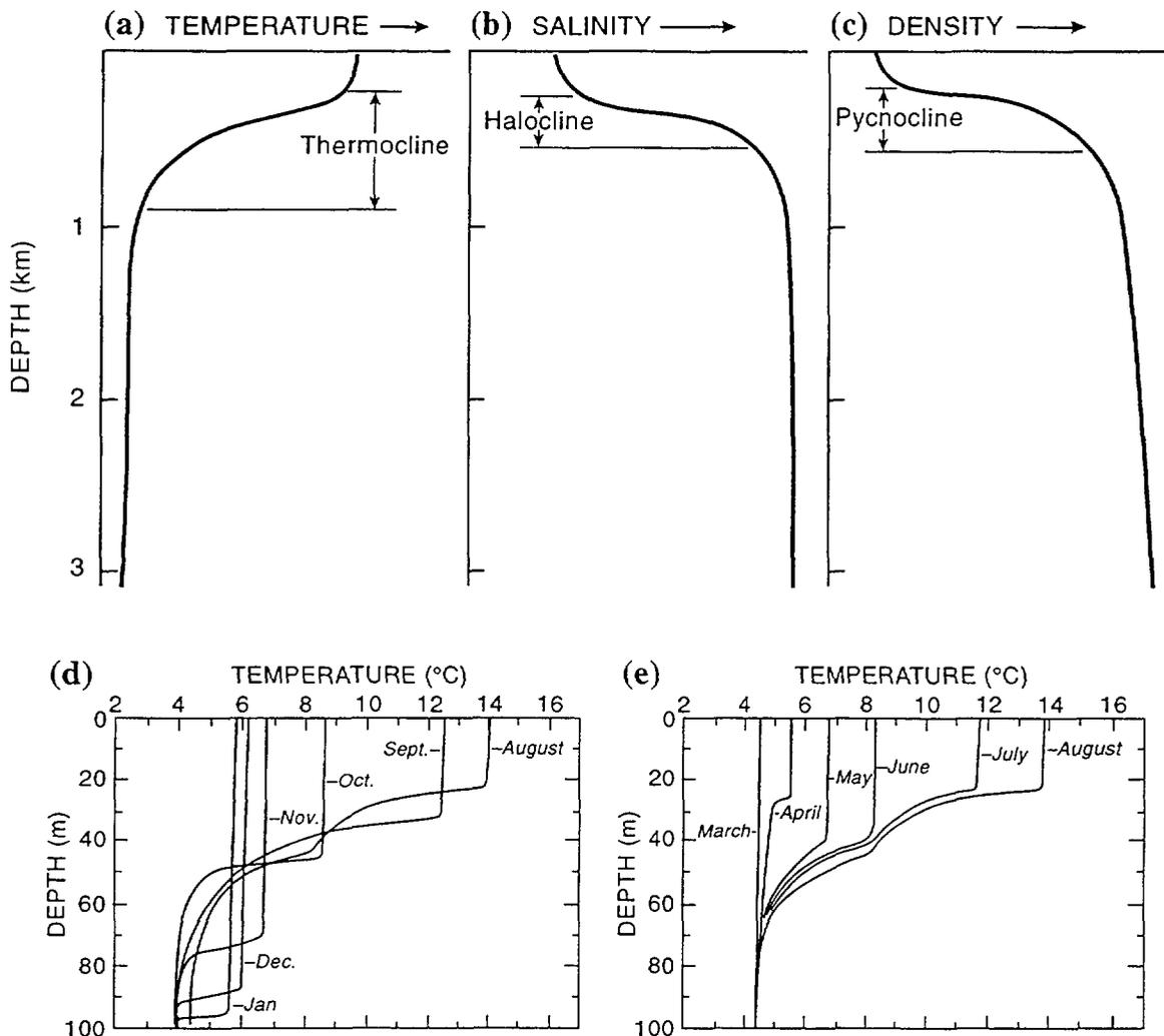
FIG. 13. Schematic representation of a thermocline (a), halocline (b), pycnocline (c), fall-winter decay of a thermocline (d), and spring-summer establishment of a thermocline (e).
