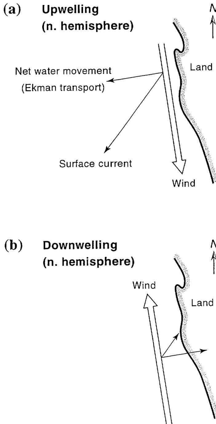
*FIG. 7. Schematic representation of coastal upwelling (a) and downwelling (b) in the northern hemisphere. The directions of the surface current and Ekman transport relative to wind direction would be reversed in the southern hemisphere, for both upwelling and downwelling events.*
