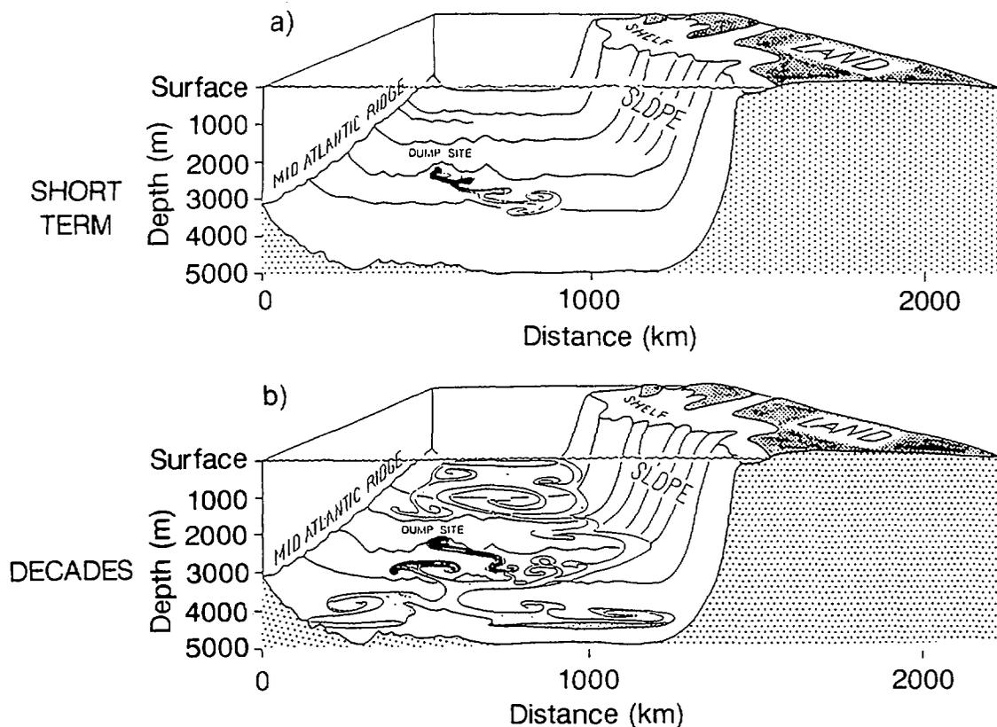
FIG. 21. Schematic diagram of the plume of contaminated seawater developing from the release of radionuclides from packaged radioactive wastes dumped in the deep ocean.
