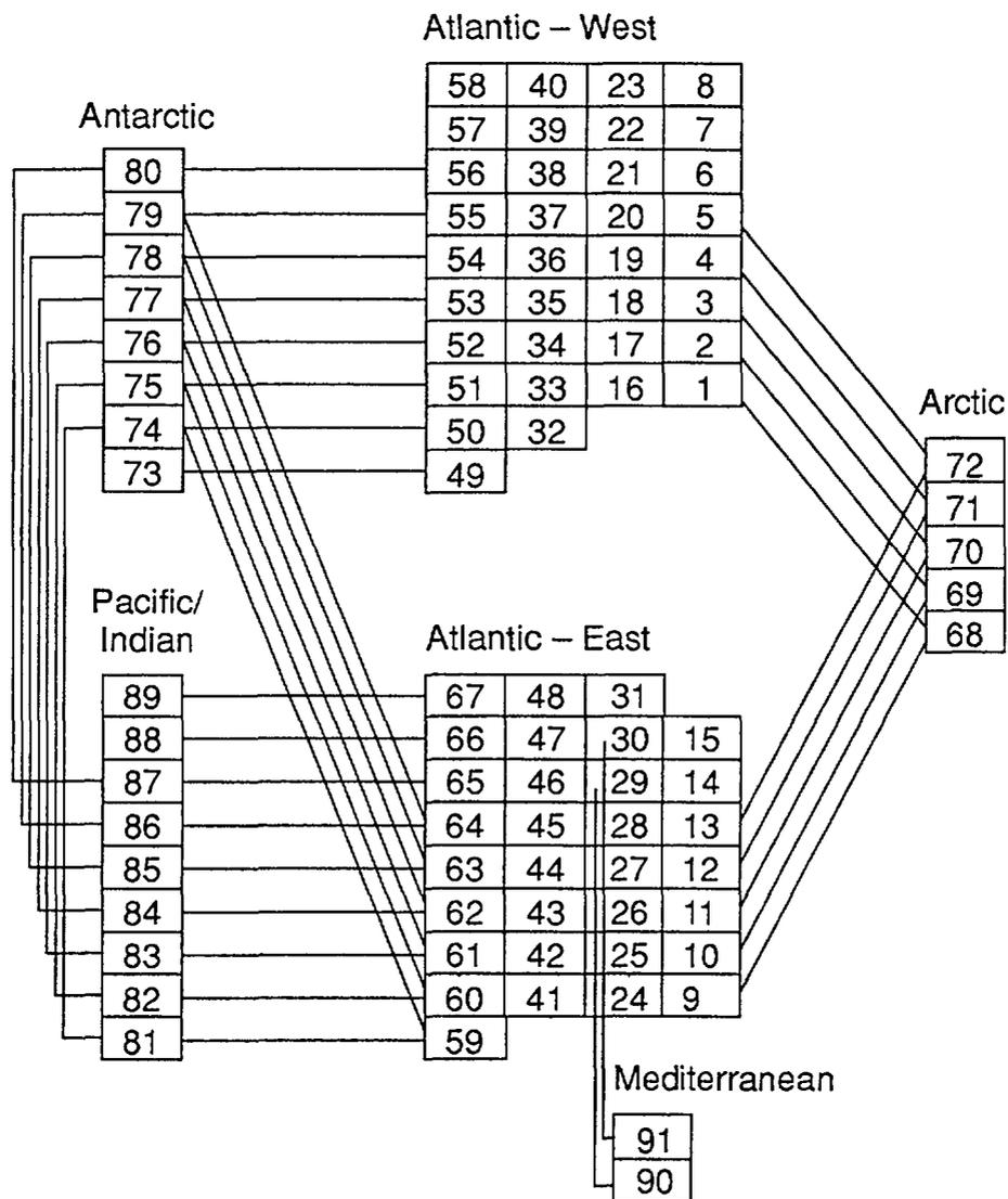
FIG. 24. The box structure used to model the wider dispersion of waste radionuclides in the world ocean. Reproduced with permission from: *Review of the continued suitability of the dumping site for radioactive waste in the North-East Atlantic*, OECD/NEA, Paris, 1985.
