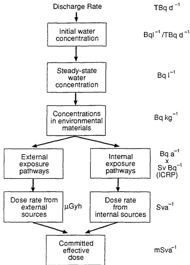
FIG. 6. Conceptual basis for undertaking a pre-operational assessment to develop an authorization for liquid radioactive waste disposal to an aquatic system.
