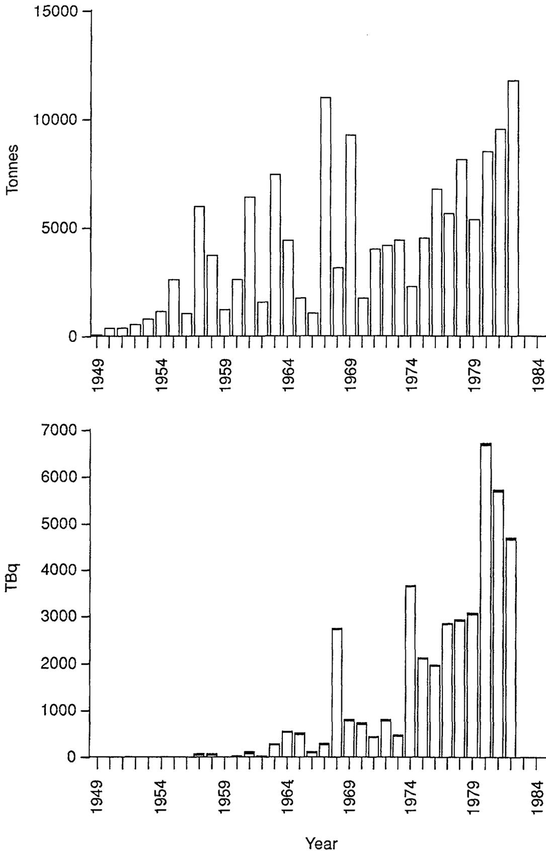
FIG. 28. Estimated total mass of the packages, and the quantities of  $\alpha$ -emitting and  $\beta/\gamma$ -emitting (excluding tritium) radionuclides dumped into the NE Atlantic Ocean each year. Adapted from: Review of the continued suitability of the dumping site for radioactive waste in the North-East Atlantic, OECD/NEA, Paris, 1985.
