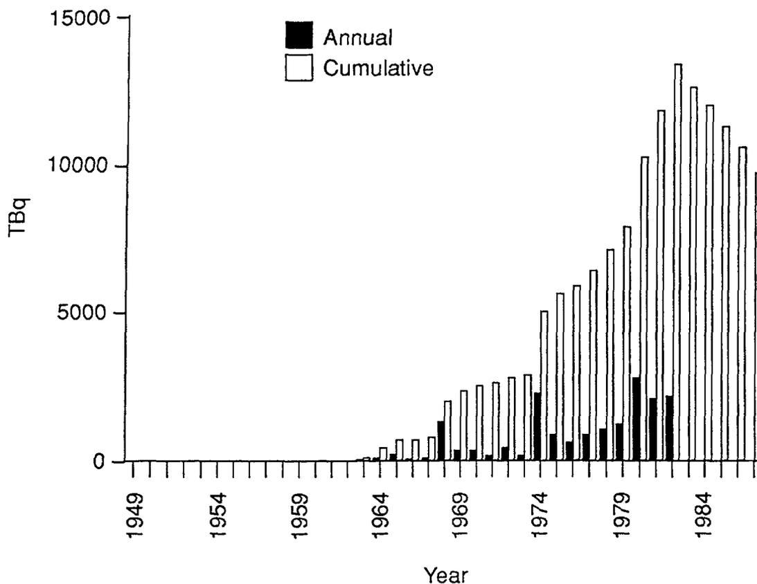
FIG. 29. Estimated annual inputs and decay-corrected cumulative environmental inventory of tritium in the NE Atlantic Ocean from packaged waste dumping. Adapted from: *Review of the continued suitability of the dumping site for radioactive waste in the North-East Atlantic, OECD/NEA, Paris, 1985.*
