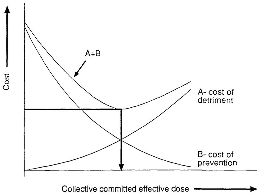
FIG. 4. A schematic example of the principle of optimization through the minimization of the aggregate costs of radiation protection and the residual detriment.
