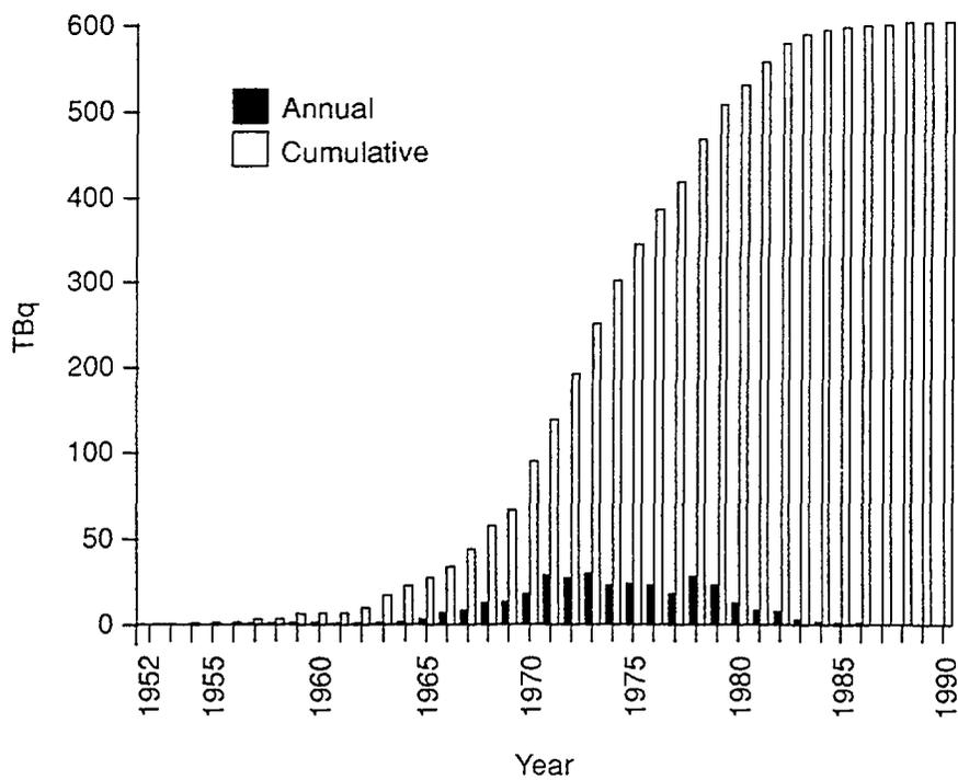
FIG. 10. Sellafield discharges to the NE Irish Sea: Annual input and cumulative decay-corrected environmental inventory of Pu-239+240.
