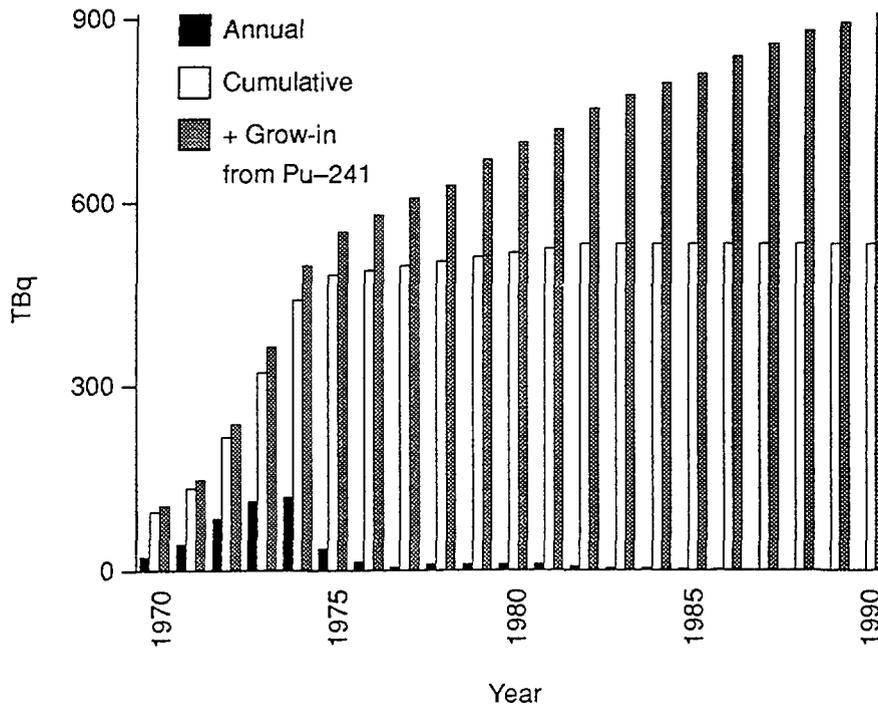
FIG. 13. Sellafield discharges to the NE Irish Sea: Annual input and cumulative decay-corrected environmental inventory of Am-241 from the annual input; and total cumulative decay-corrected environmental inventory of Am-241 including in-growth from the decay of the environmental inventory of Pu-241.
