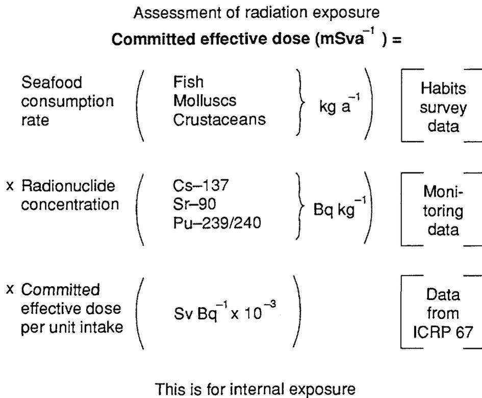
FIG. 14. Procedure for assessing the radiation exposure from internal sources arising from the consumption of contaminated seafood.
