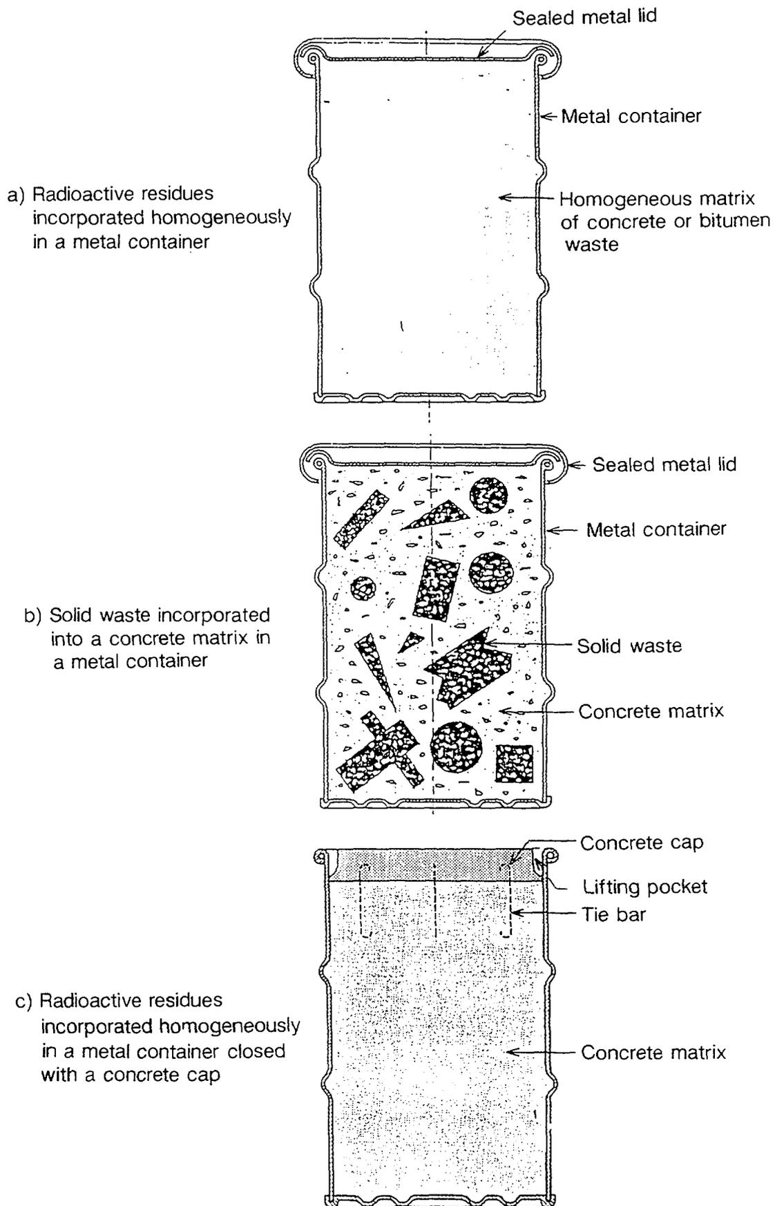
FIG. 26. Approved waste package designs used as a basis for modelling the release of radionuclides to seawater.
