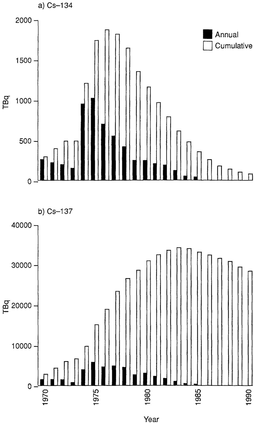
FIG. 8. Sellafield discharges to the NE Irish Sea: Annual inputs and cumulative decay-corrected environmental inventories of Cs-134 and Cs-137.
