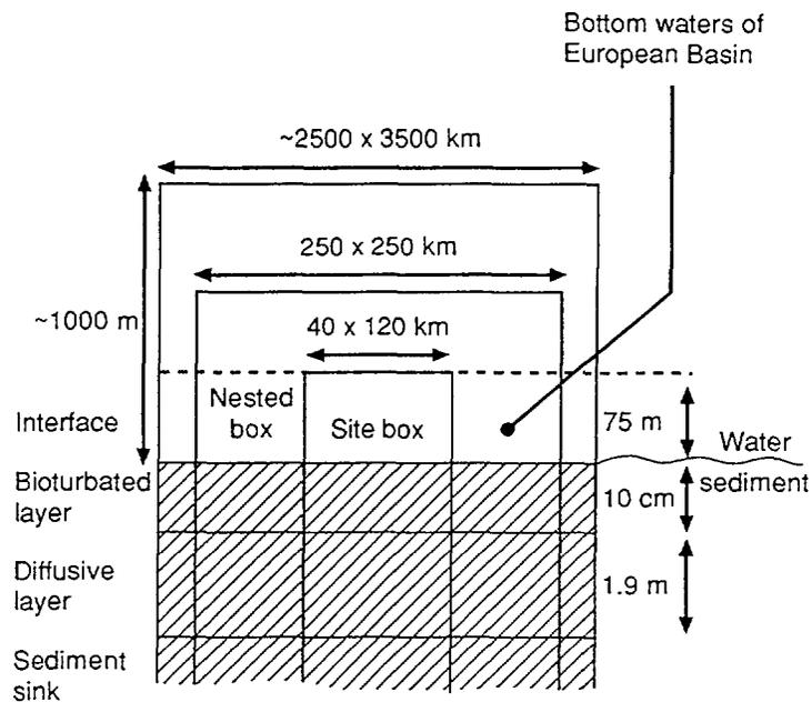
FIG. 23. The nested box structure around the dump site used to model the initial dispersion of radionuclides released from the wastes. Reproduced with permission from: Review of the continued suitability of the dumping site for radioactive waste in the North-East Atlantic, OECD/NEA, Paris, 1985.
