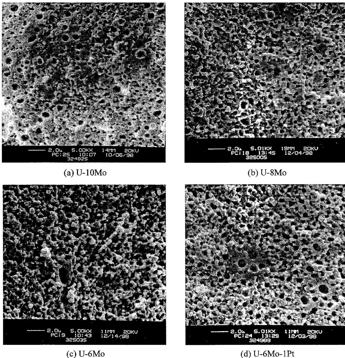
Fig. 3. Scanning electron micrographs of typical portions of fuel particles from various U-Mo alloys at approximately 70% burnup illustrating similar behavior.
