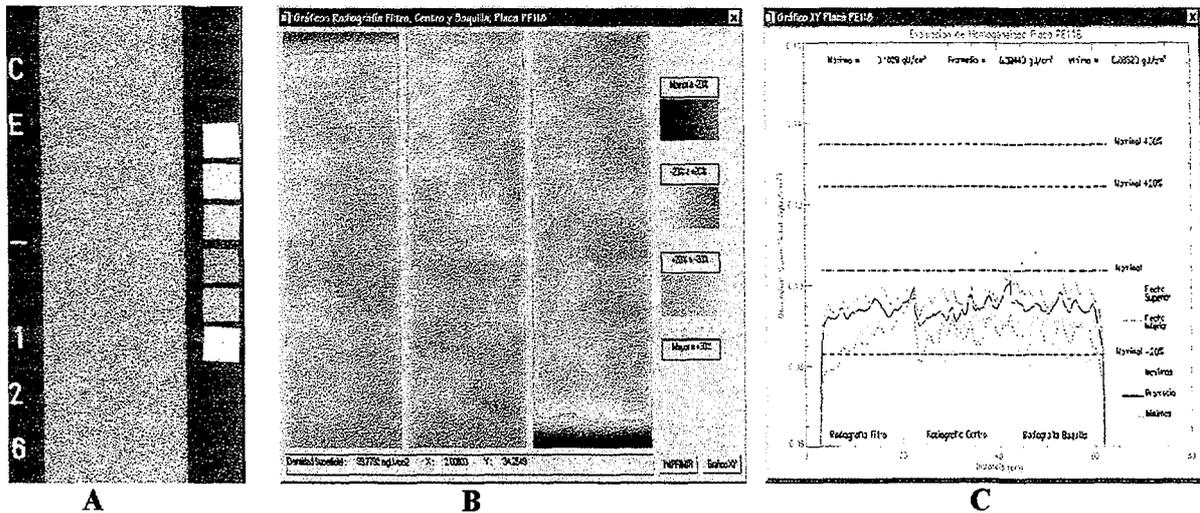
Fig. 5. Homogeneity Image Analysis. A: scanned image, B: results in image form, C: results in graph form
