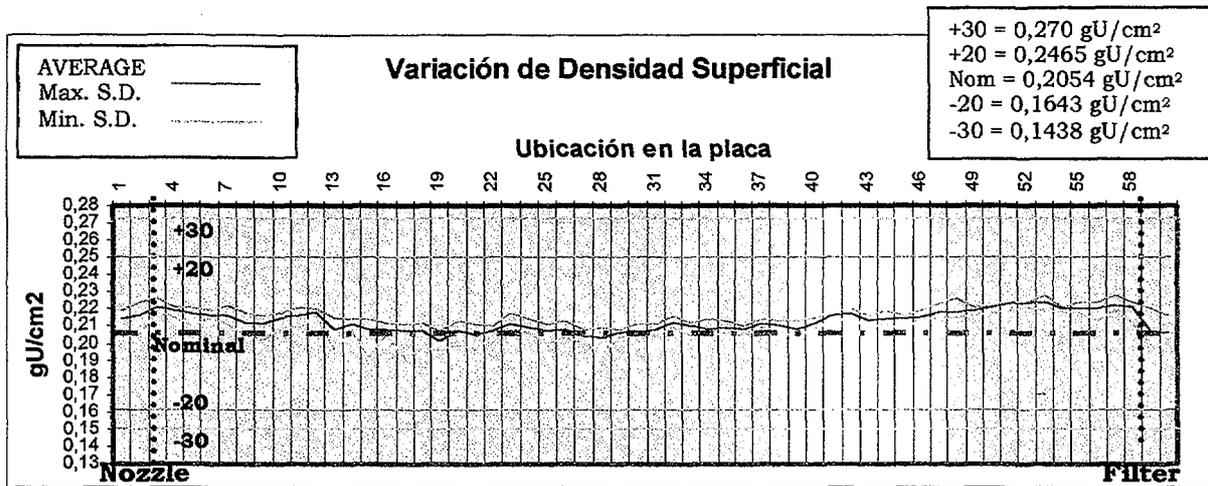
Fig. 3. Surface density graph for an internal fuel plate
