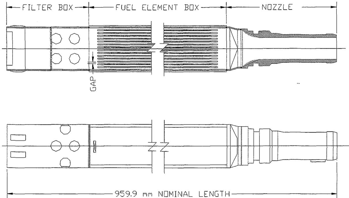
Fig. 1 Sketch of the RECH-1 Fuel Element.
