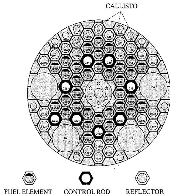
Fig. 1 Horizontal cross-section at reactor mid-plane of a typical BR2 loading, with three channels containing CALLISTO rigs.
