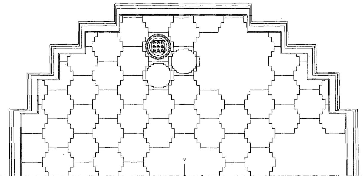
Fig. 4 (X,Y)-geometry model of BR2 for the DORT calculations with CALLISTO in channel K49
