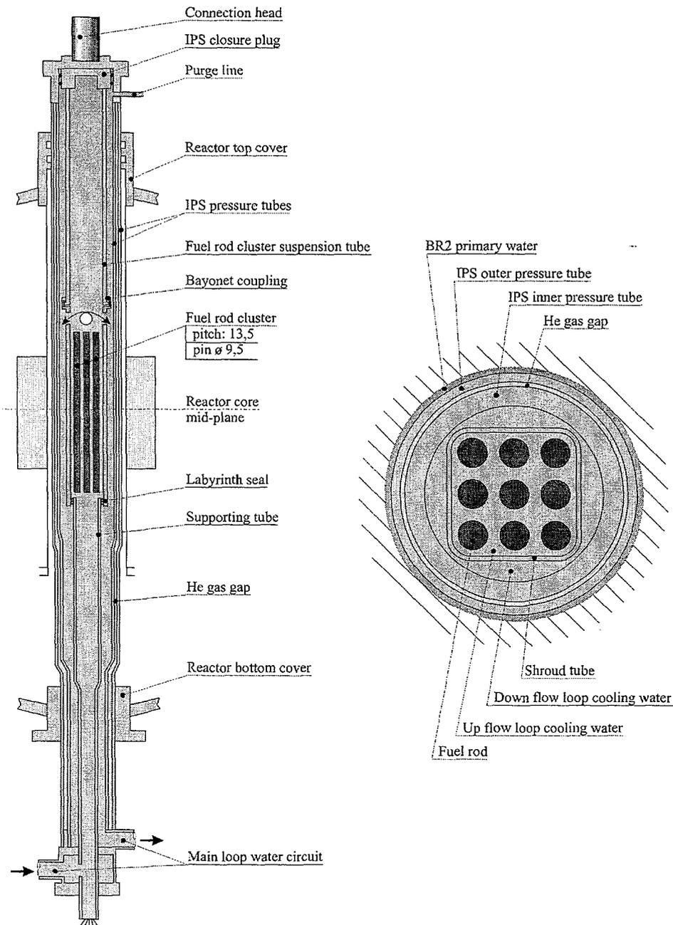
Fig. 2 Horizontal and vertical cross-sections of the CALLISTO irradiation facility
