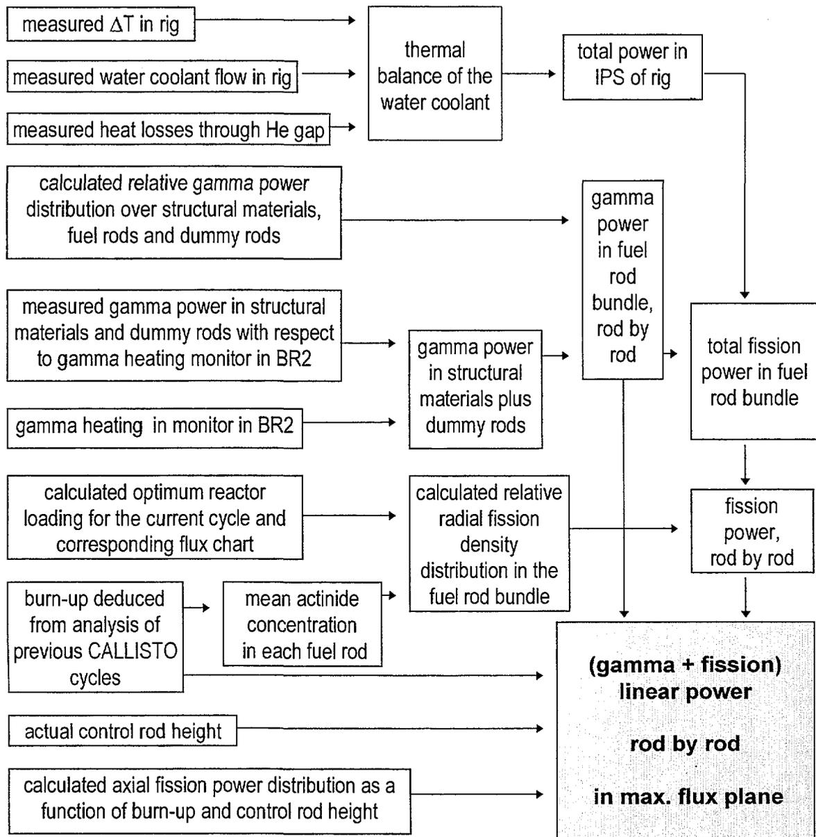
Fig. 3 Flow chart of the procedure for the accurate determination of the linear powers in the nine fuel rods of a CALLISTO rig
