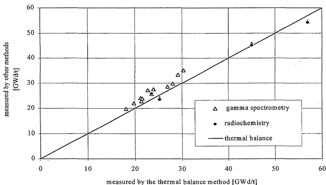
Fig. 6 Peak burn-up determination of the fuel rods in CALLISTO: comparison of the results obtained by various methods
