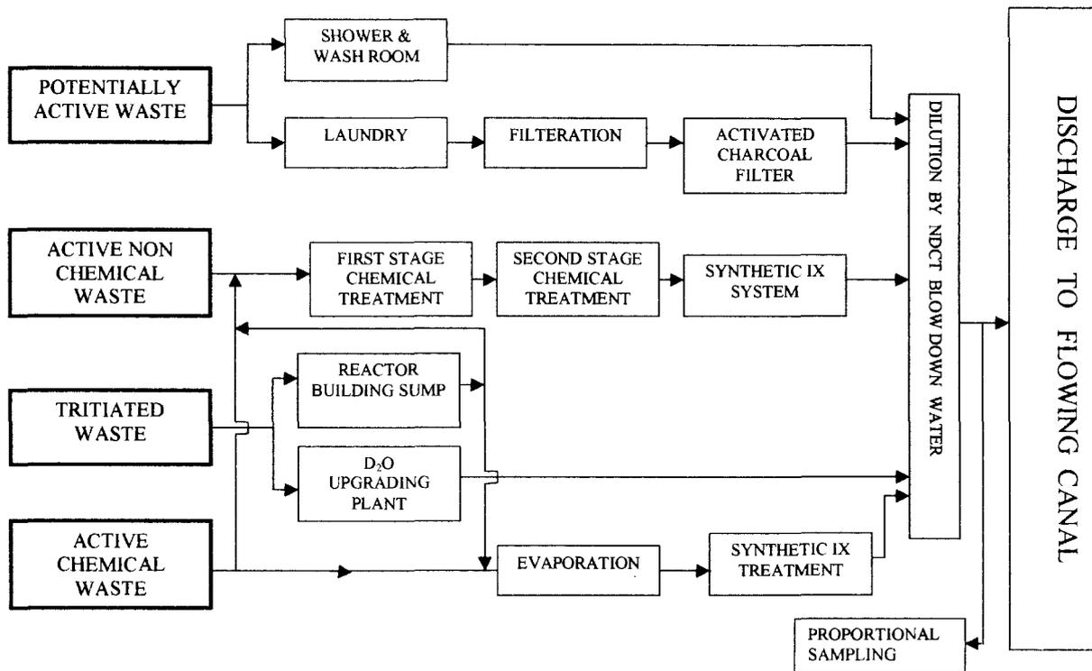
FIG. 1. Liquid waste treatment and disposal schematic.
