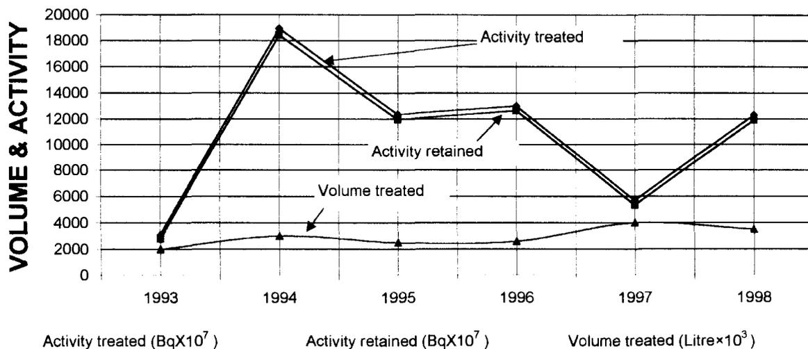
FIG. 2. Performance of chemical treatment system.
