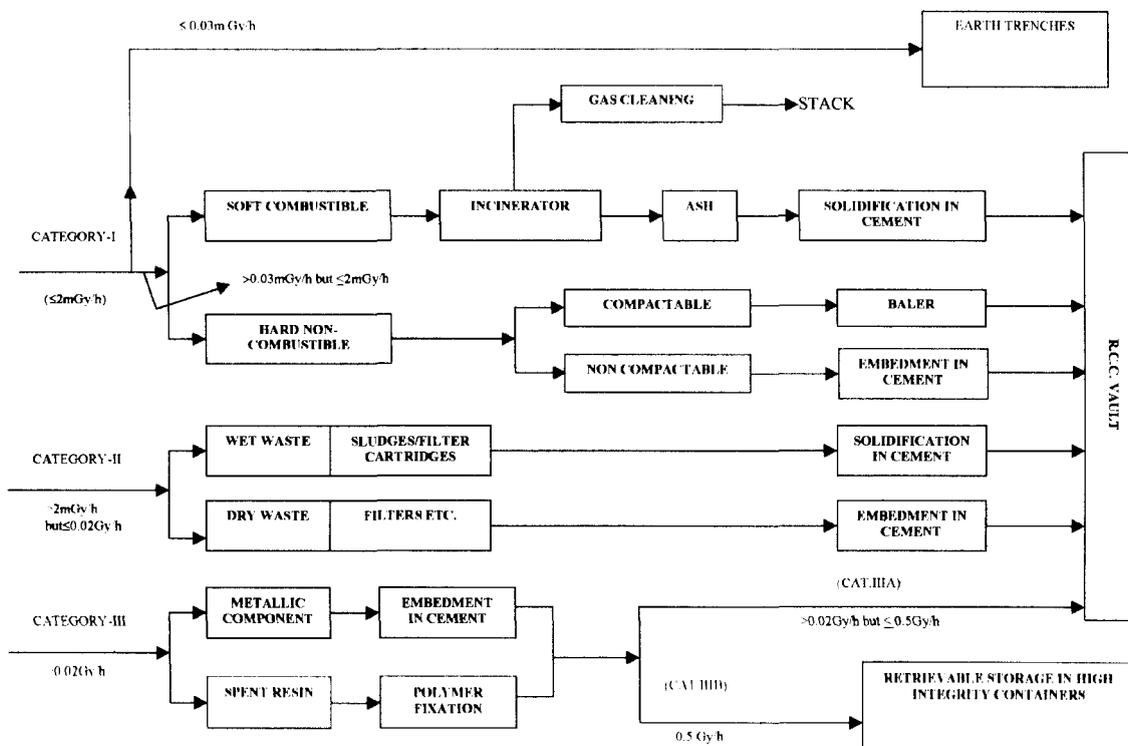
FIG. 3. Solid waste conditioning & disposal schematic.
