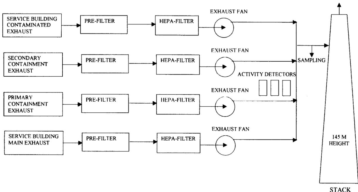
FIG. 5. Gaseous effluent management schematic.
