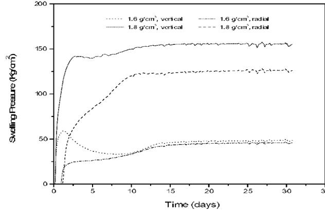
Fig. 1. Development of swelling pressure versus elapsed time for bentonite.
