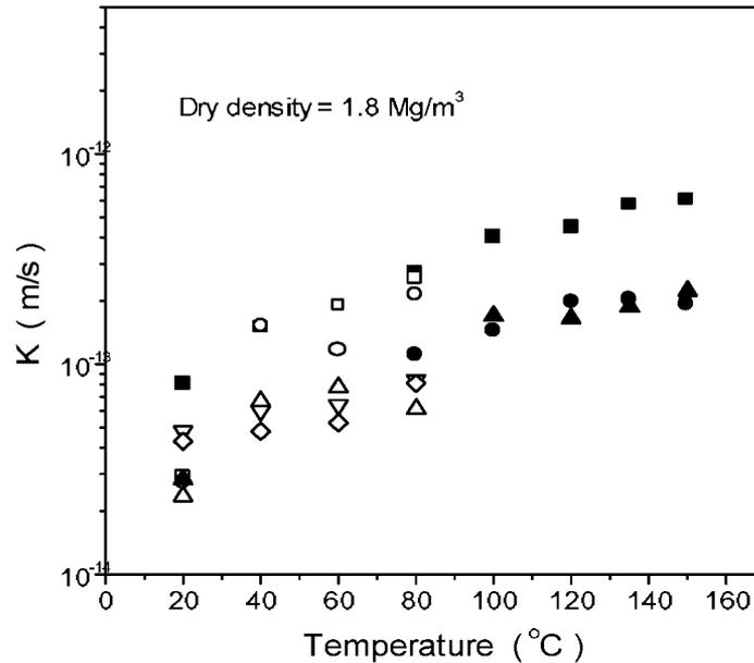
Fig. 7. Influence of temperature elevation on the hydraulic conductivity of compacted bentonite.
