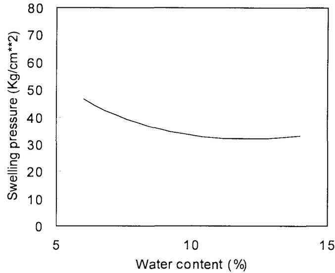
Fig.5. Effect of initial water content on the swelling pressure for bentonite (dry density=1.6 Mg/m<sup>3</sup>).
