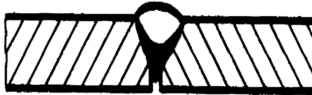
FIG. 10. Incomplete root penetration.
