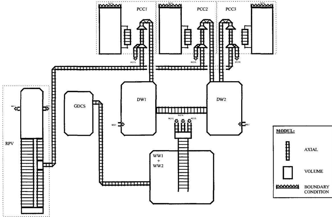
FIG.1. Nodalization of phase A (PANDA — CATHARE nodalization).
