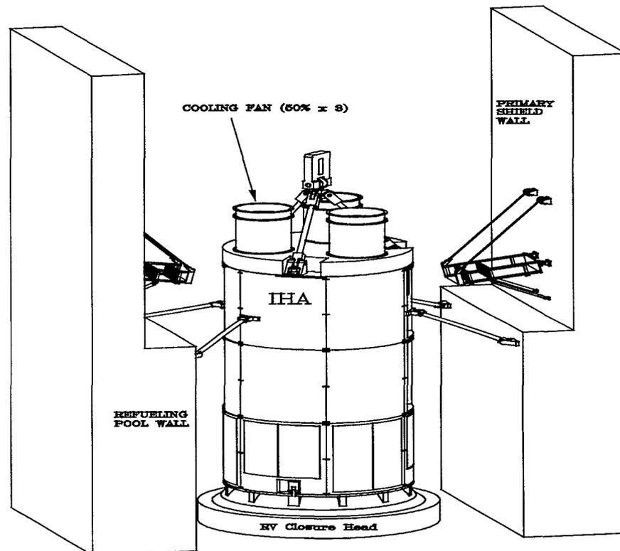
FIG. 2. Integrated head assembly (IHA) for KNGR.
