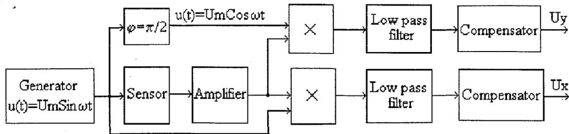
Fig. 2. The functional scheme of electronic compensation
