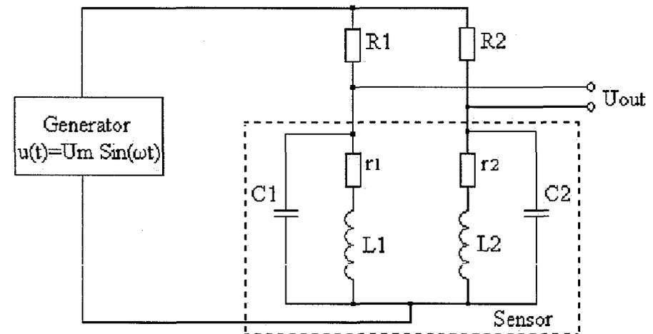
Fig. 1. Scheme connection of sensor
