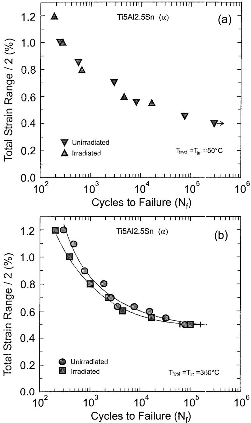
Figure 18. Fatigue lives of the  $\alpha$ (Ti5Al2.5 Sn) titanium alloy determined at 50 and 350°C in the unirradiated and irradiated conditions.
