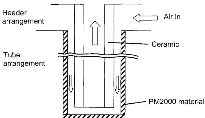
**Figure 3. ODS bayonet tube arrangement.**
