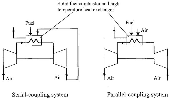
**Figure 2. Different layouts of indirectly fired gas turbines.**
