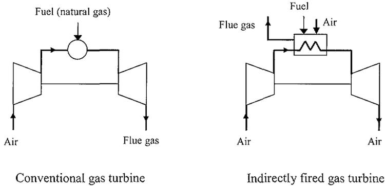
**Figure 1. Conventional and indirectly fired gas turbines.**
