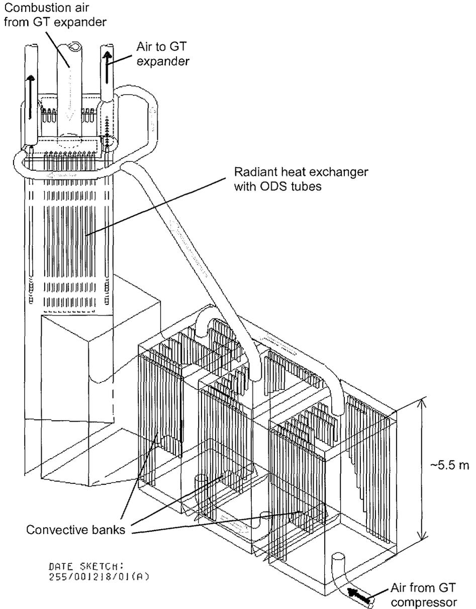
Figure 4. Layout of high temperature heat exchanger.
