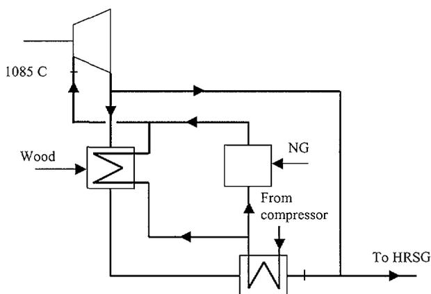
Figure 6. Integration of a natural gas fired topping combustor.
