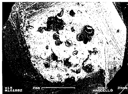
Fig. 7 Longitudinal section of the composite sintered bronze 4 wt% \phi = 5.00 mm diamond
