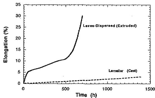
Figure 6 – Creep results for Cr-Ta alloys. Note that the as-cast material with a lamellar structure showed very little elongation during the test run at 1000°C and 138 MPa in humid air. The composition of the alloy was Cr-8Ta-5Mo-0.5Ti-0.01Ce. Figure courtesy of Dr. Michael Brady of Oak Ridge National Labs.
