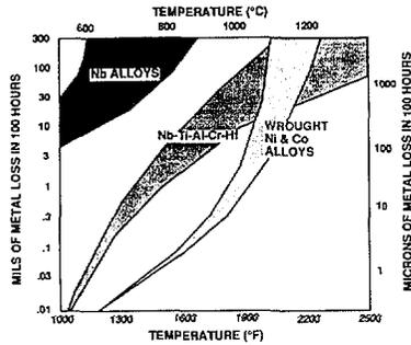
Figure 5 – A comparison of the oxidation of Nb-based material with the oxidation of Ni- and Co-based superalloys. Note that the addition of Ti, Hf, and Al greatly reduces the oxidation rate over that for monolithic Nb alloys that do not contain these additions. Figure courtesy of Dr. M.R. Jackson of the General Electric Research and Development Center.
