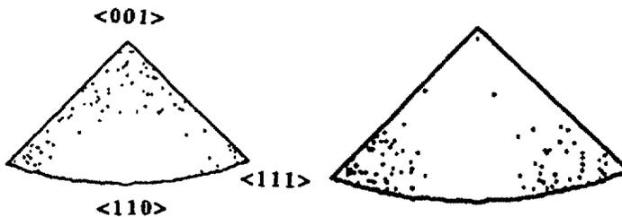
Figure 8 – Inverse pole figures for rolled and recrystallized tantalum. (a.) The inverse pole figure for a sample rolled to 2.8 mm and recrystallized. (b.) The inverse pole figure for a sample rolled to 0.13 mm and recrystallized. In both cases the direction of the inverse pole figure was that perpendicular to the rolling surface. Note that with continued deformation and recrystallization, the texture becomes strongly  $\langle 110 \rangle$ .
