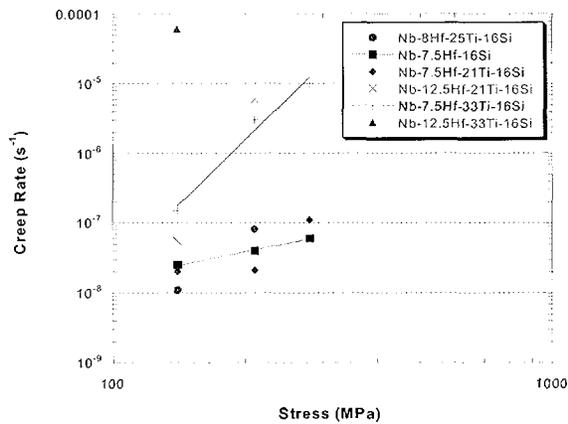
Figure 4 – Creep rates of five Nb-silicide based in situ composites. The samples were tested in compression at  $1200^{\circ}C$ . Note that additions of Ti and Hf above 25 and 8%, respectively, causes the creep rate to increase significantly. Data taken from reference 13.
