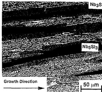
Figure 3: The microstructure of a niobium silicide in-situ composite prepared by directional solidification. Micrograph courtesy of B.P. Bewlay of the General Electric Company.
