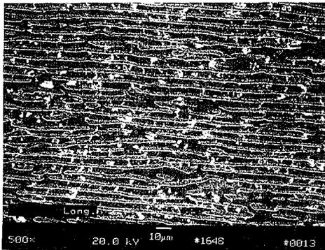
Figure 2 – Microstructures prepared by the optical imaging float zone furnace. The microstructure is from a 44Nb-54Cr alloy. The lighter phase is the Nb solid solution. The micrograph is taken parallel to the growth direction of the composite. Figure taken from Reference 11.
