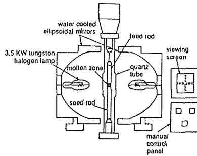
Figure 1 – A schematic of the optical imaging float zone furnace used for directional solidification of refractory based materials. Figure taken from reference 11.
