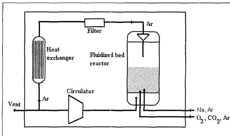
Schematic design of the sodium treatment process
