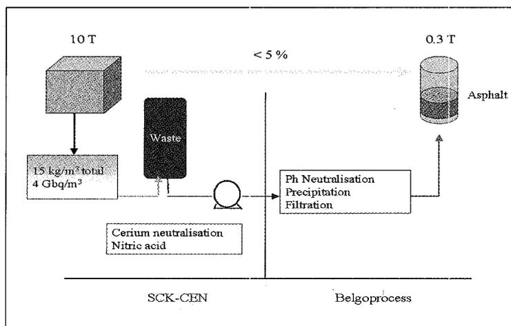
*Secondary waste removal and treatment routes for the MEDOC decontamination installation.*
