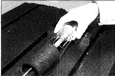
*RIED ceramics samples with their wiring and heating part*
