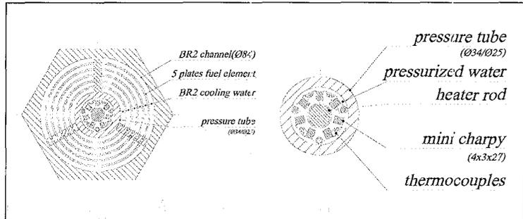
*Cross section of the MISTRAL irradiation device installed in a BR2 5 plates fuel element*
