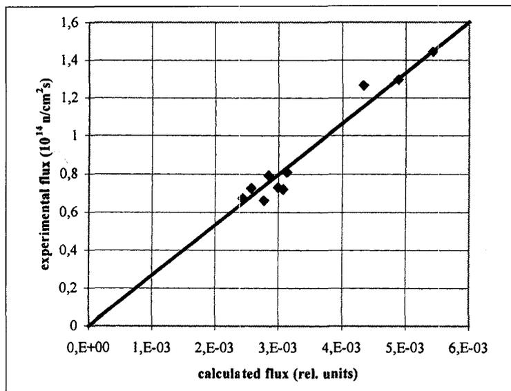
*Results for the 11 SPND's in DOLMEN during the BR2 cycle 05/2000: conventional thermal neutron fluxes obtained from the observed detector currents combined with the calculated detector sensitivities vs. the calculated relative neutron flux at the detector positions.*
