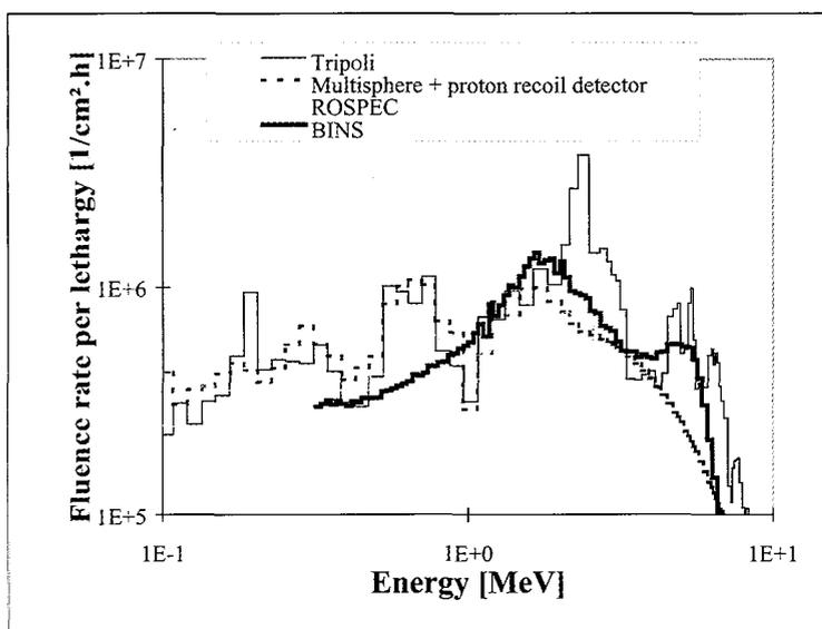
The neutron spectrum around the Venus reactor determined by four different methods.
