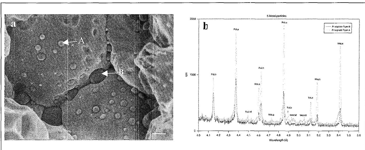
(a) Intergranular Decohesion Of Spent Fuel Sample Showing Large Metallic Precipitates On Grain Boundaries. Although The Morphology Of The Precipitates Is Different, Their Chemical Composition Seems To Be Identical (b).
