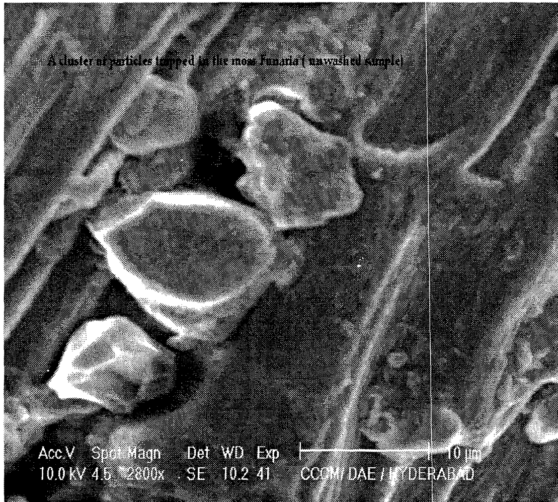
Fig.2. SEM image of soil particles trapped in a Funaria moss sample.
