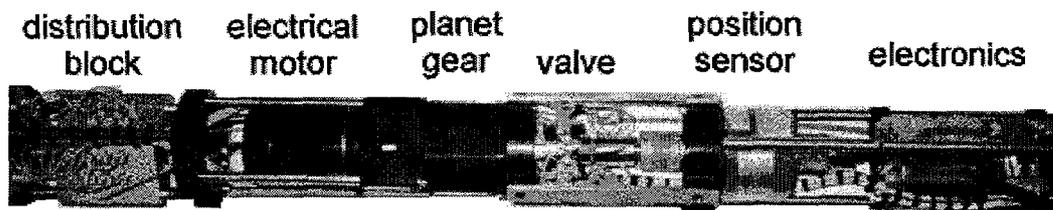
Figure 1-1. One of six multi-channel valves in CHEMLAB.
