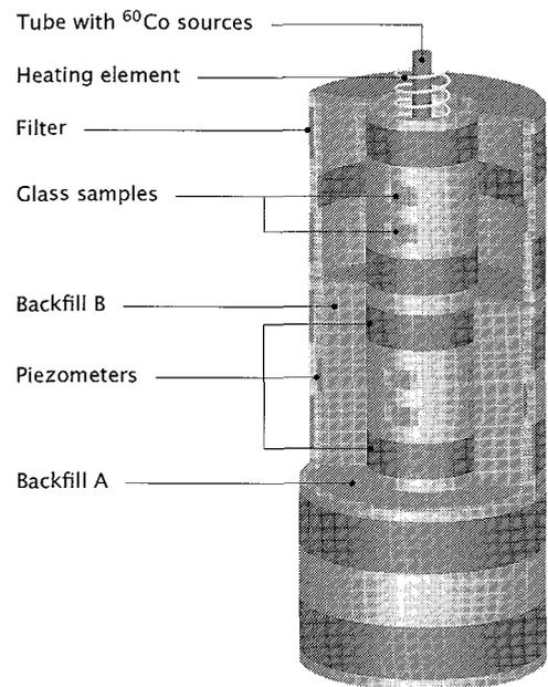
**Figure 4** Three-dimensional view of a CORALUS test tube. Backfill and outer porous support tube of modules B and C are cross-sectioned to show details of the inner support tube.
