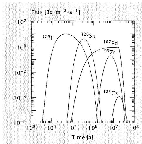
**Figure 1** Calculated fluxes of selected radionuclides released from the host clay layer into the Neogene aquifer.
