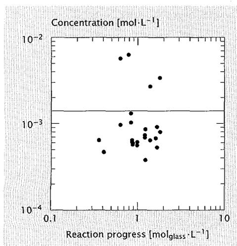
**Figure 2** Measured (points) and calculated (line) concentrations of silicon released from the SON68 glass in a Boom Clay / clay-water slurry, at 90°C.
