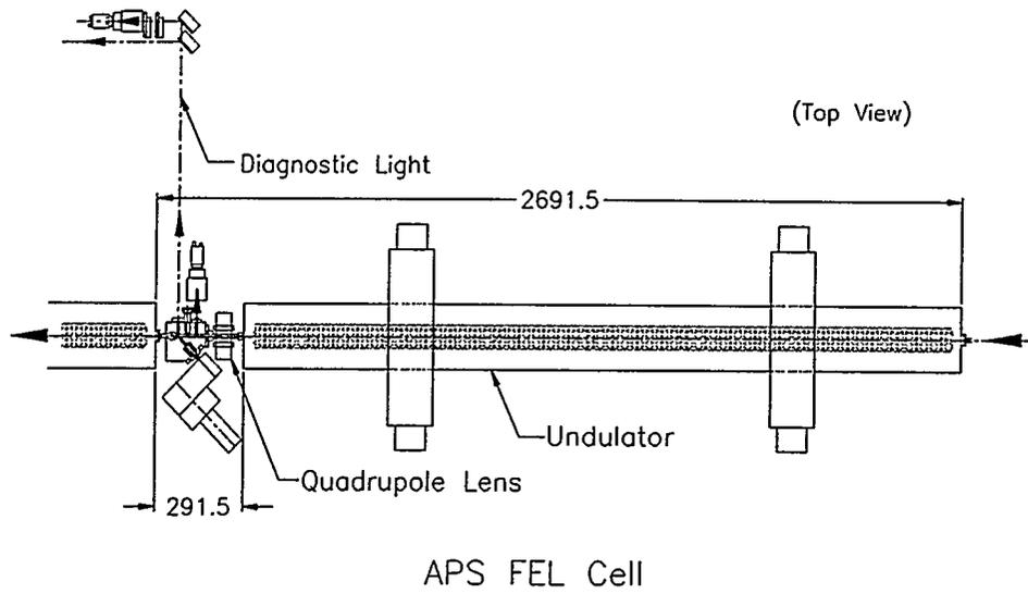
Figure 6: APS SASE FEL undulator cell.
