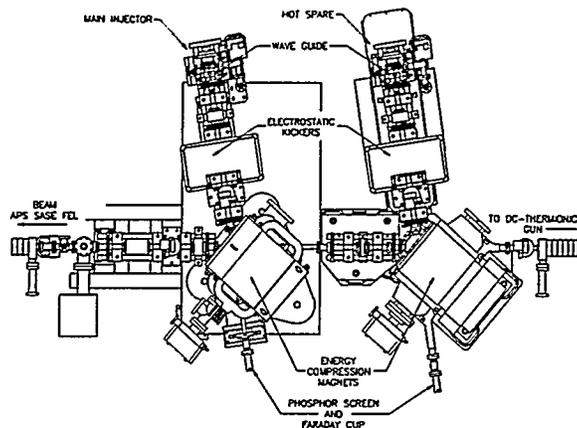
**Figure 2:** The APS linac front end with the two thermionic rf guns and compression magnets.
