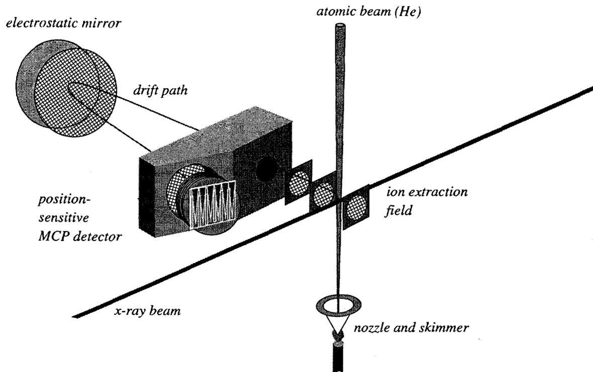
Figure 5: Schematic of the time-of-flight spectrometer.
