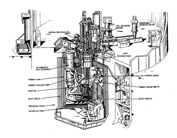
Fig. 1. EBR-II Reactor and Primary System
