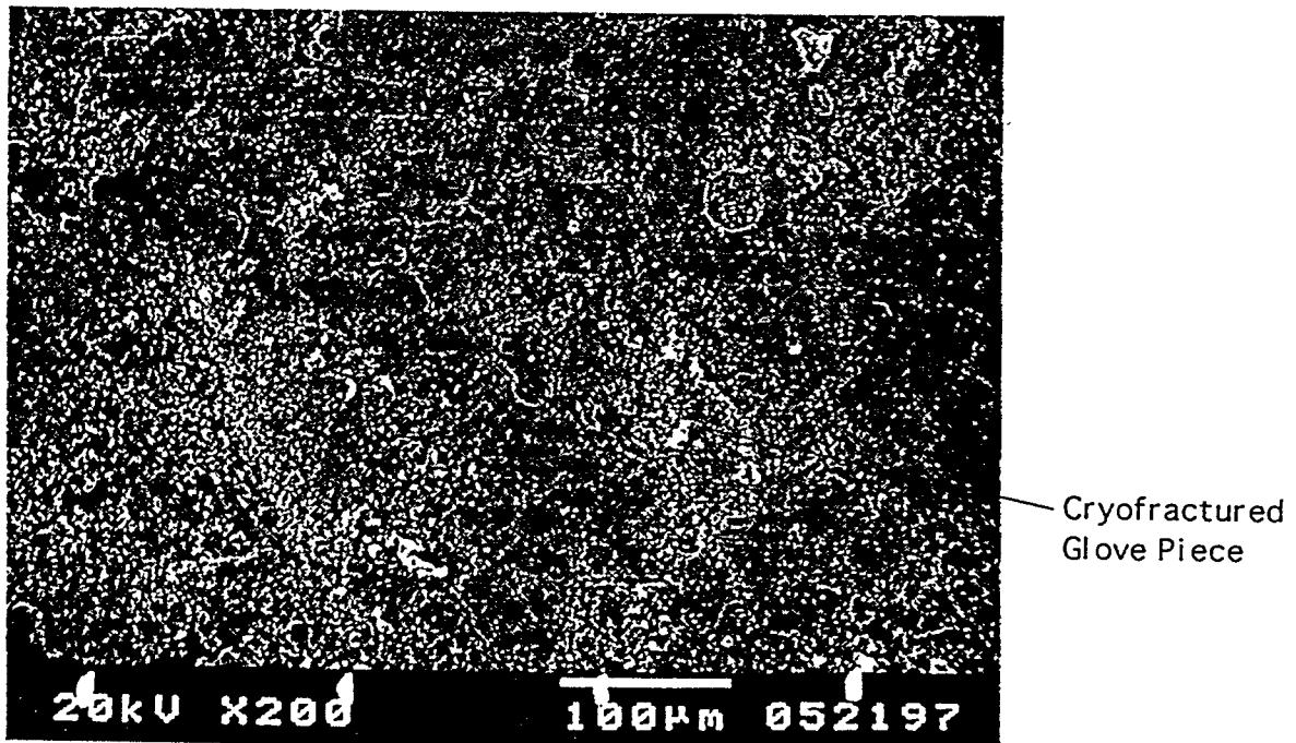
Fig. 4. Photomicrograph of MKP-35 wt.% cryofractured plastic glove waste form.
