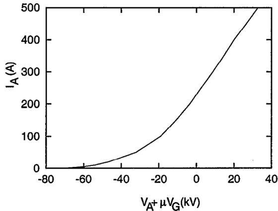
Figure 2: Anode current versus effective voltage for a screen voltage of 2 kV. The amplification factor is  $\mu = 132$
