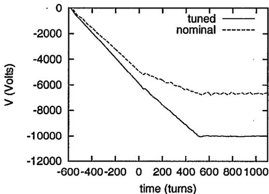
Figure 6: In phase amplitude of gap voltage ( $I_g$ ) during the cycle for the nominal case and with dynamic tuning.
