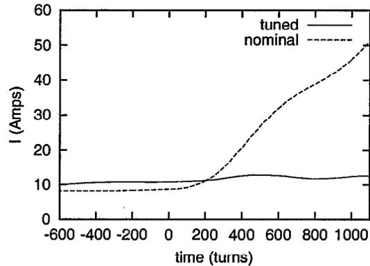
Figure 7: DC anode current during the cycle for the nominal case and with dynamic tuning.
