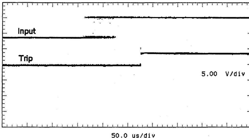
FIGURE 5. Response time measurement with a step input. The measurement shows a best case of 52  $\mu s$  and a worst case of 113  $\mu s$ . The figure shows 500 traces overlaid.
