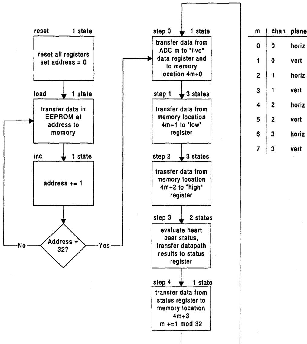
FIGURE 4. Controller state diagram.
