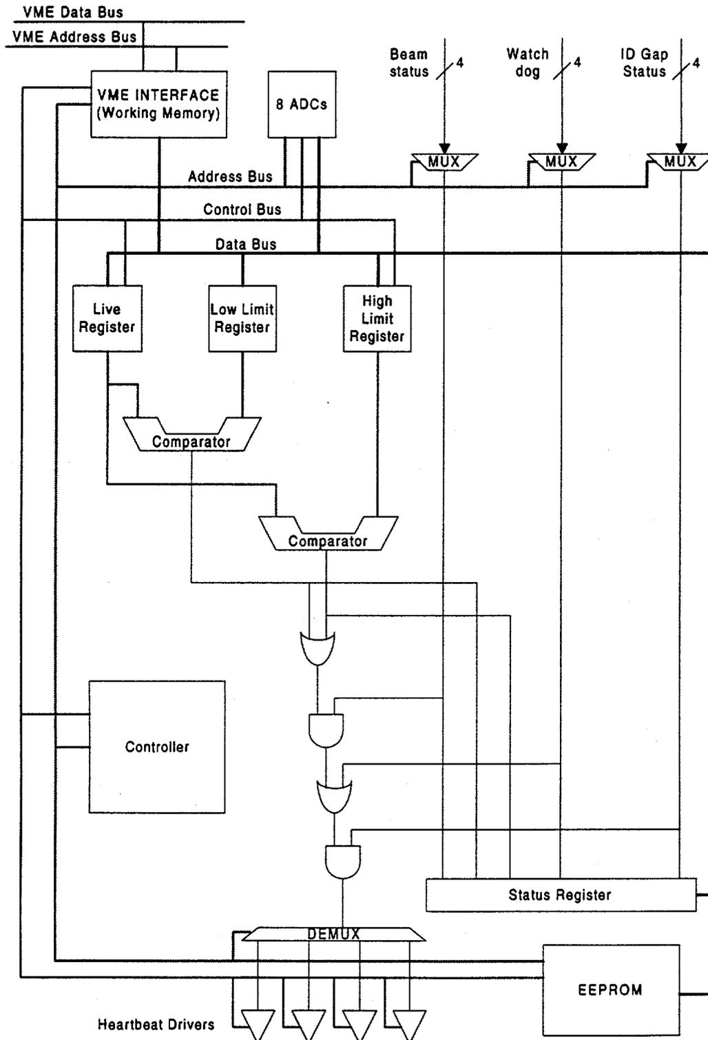
FIGURE 2. Block diagram of DBPLD internals.
