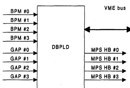
**FIGURE 1.** DBPLD inputs and outputs. One DBPLD board supports four BPMs that cover two insertion devices. Insertion device gap open/closed status is sensed through the GAP inputs. An optical heartbeat (MPS HB) is sent to the machine protection system when no missteering condition exists. The DBPLD is interfaced to the APS control system through an onboard VME interface.
