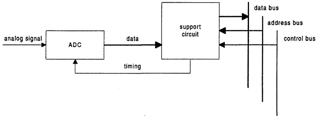
**FIGURE 3.** ADC section, analog-to-digital converter with support circuit. The support circuit simplifies timing between the ADC and the rest of the DBPLD.
