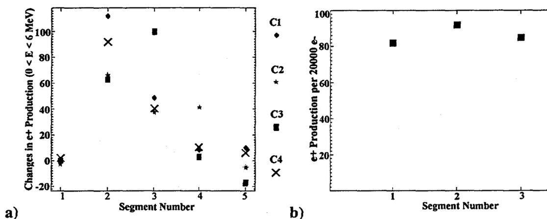
Figure 2: a) Changes in positron yield after each segment for four configurations at 400 MeV. b) Positron yield per segment for the optimized 14-MeV target, based on a).
