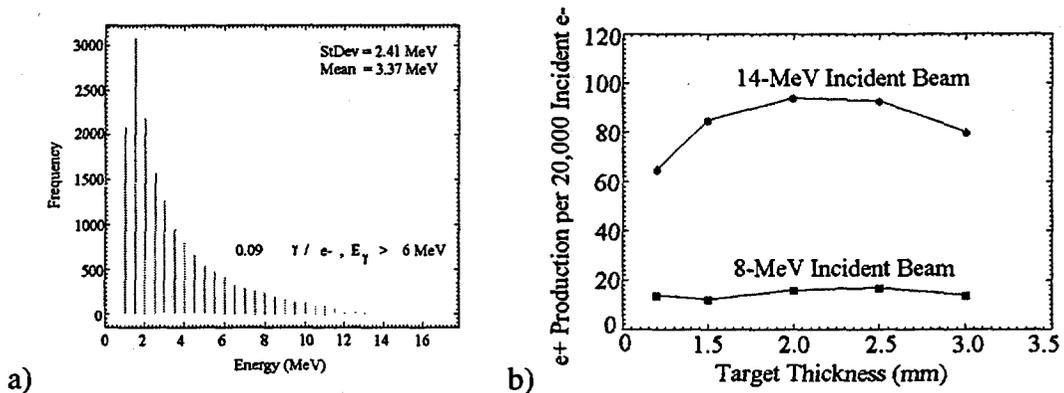
**Figure 1:** a) Photon energy distribution from 20000 14-MeV electrons impinging on a 1.2-mm tungsten target. b) Forward positron production as a function of single-block target thickness for 8- and 14-MeV electrons.
