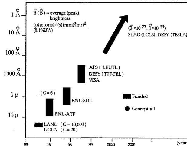
**FIGURE 2.** SASE projects around the world. The numbers within the parentheses (G=) indicate the experimentally observed gain to date.
