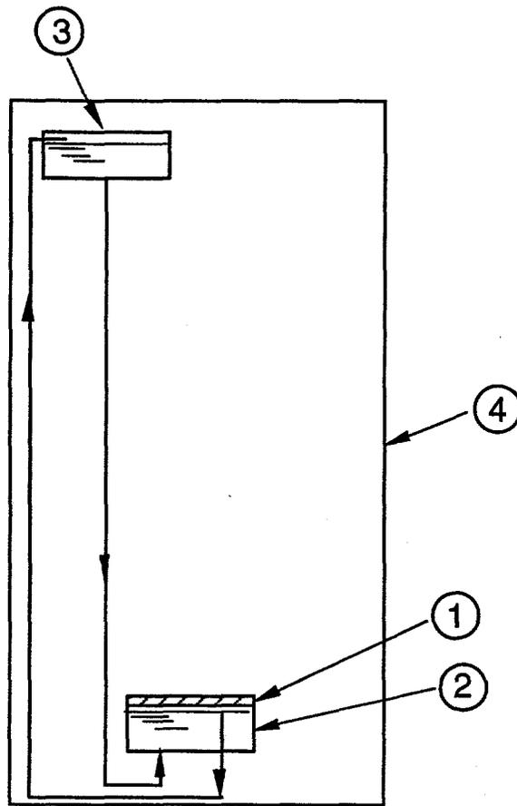
Figure 2. Liquid Bath Cooling System Schematic.
