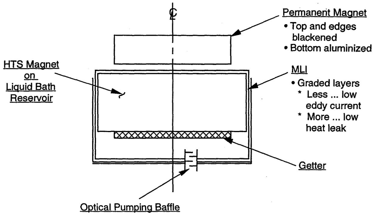
Figure 4. Thermal control and vacuum pumping
