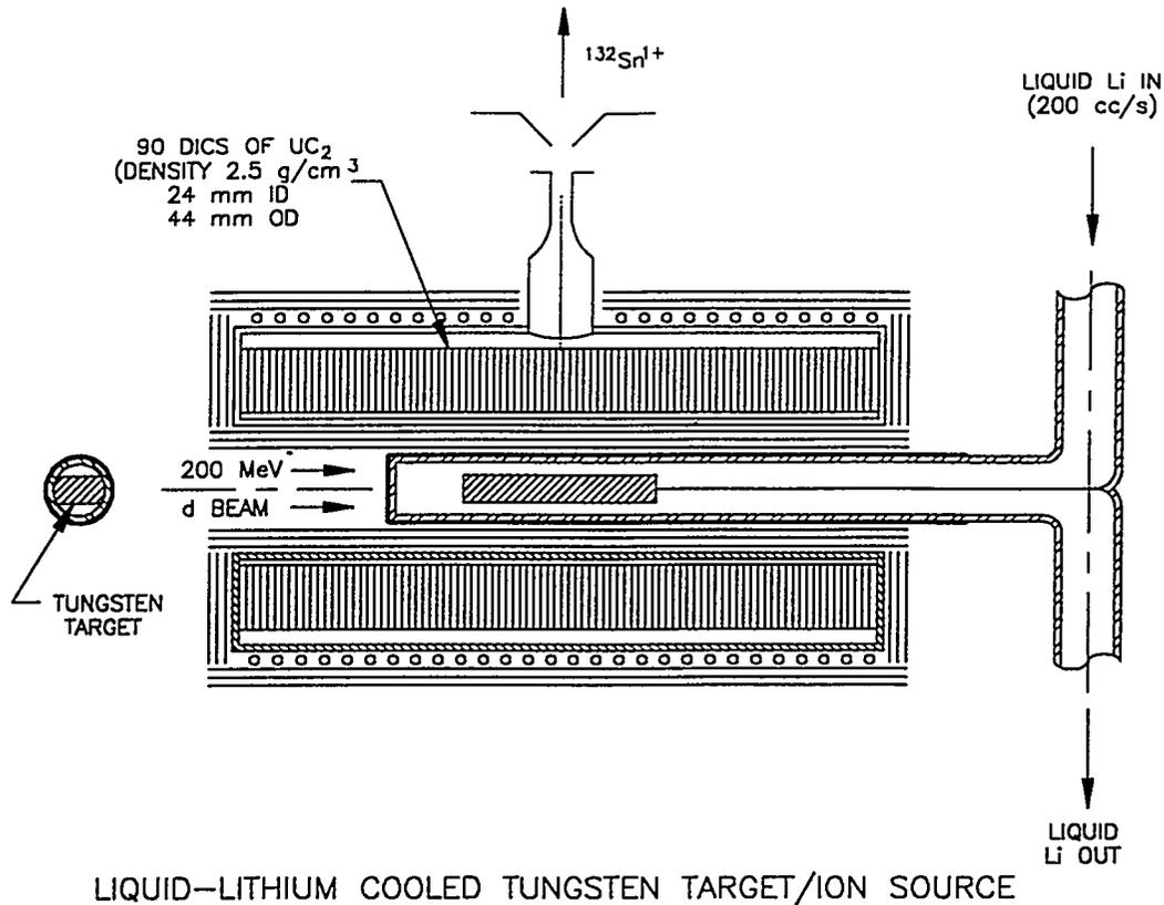
LIQUID-LITHIUM COOLED TUNGSTEN TARGET/ION SOURCE
