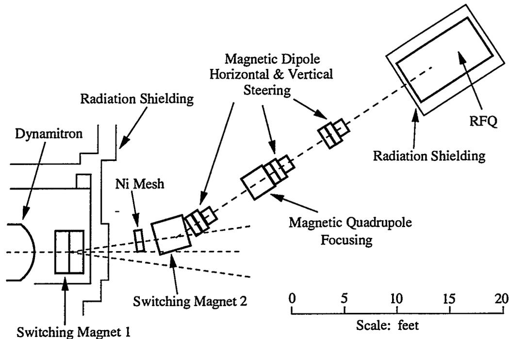
**FIGURE 1.** Schematic showing an overhead view of the current beam transport system between the Dynamitron injector accelerator and the RFQ.
