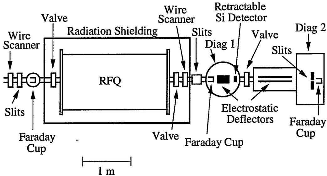
**FIGURE 2.** Schematic showing an overhead view of the proposed beam diagnostic stations used at the entrance and exit sections of the RFQ.
