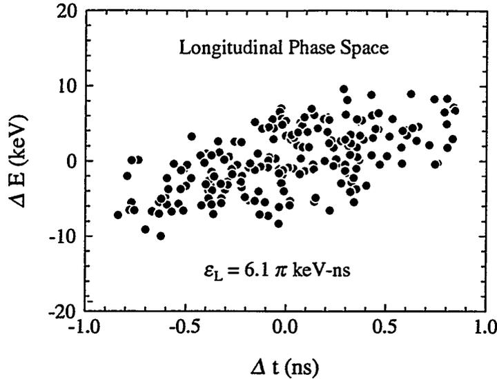
**FIGURE 4.** Numerically simulated longitudinal phase space of 200  $^{132}\text{Sn}$  ions at the exit of the RFQ [1].
