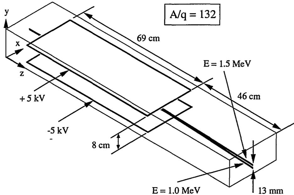
**FIGURE 3.** Results of a SIMION simulation indicating the flight paths of 1.0 MeV and 1.5 MeV beams, each having  $A/q = 132$  and diameters of 6 mm, through a potential difference of 10 kV between a pair of electrostatic deflector plates having the dimensions as indicated. The  $y$ -direction deflection difference of 13 mm refers to the centroid position of each beam.
