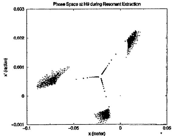
Fig 7 MAD Simulation of Beam Being Extracted at H9
