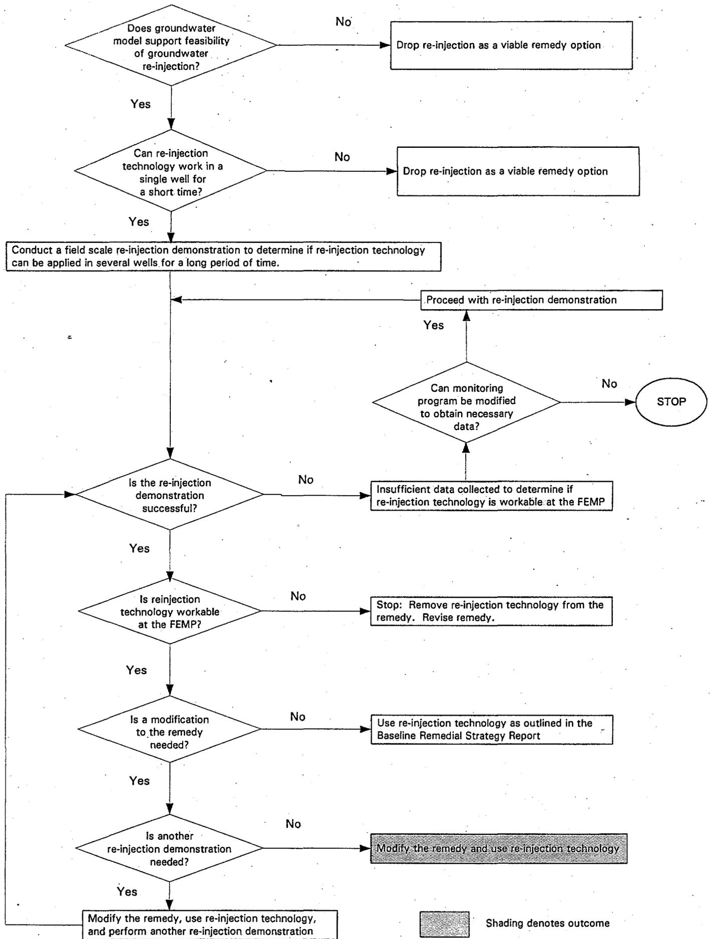
Figure 2 Re-injection Technology Evaluation Flowchart
