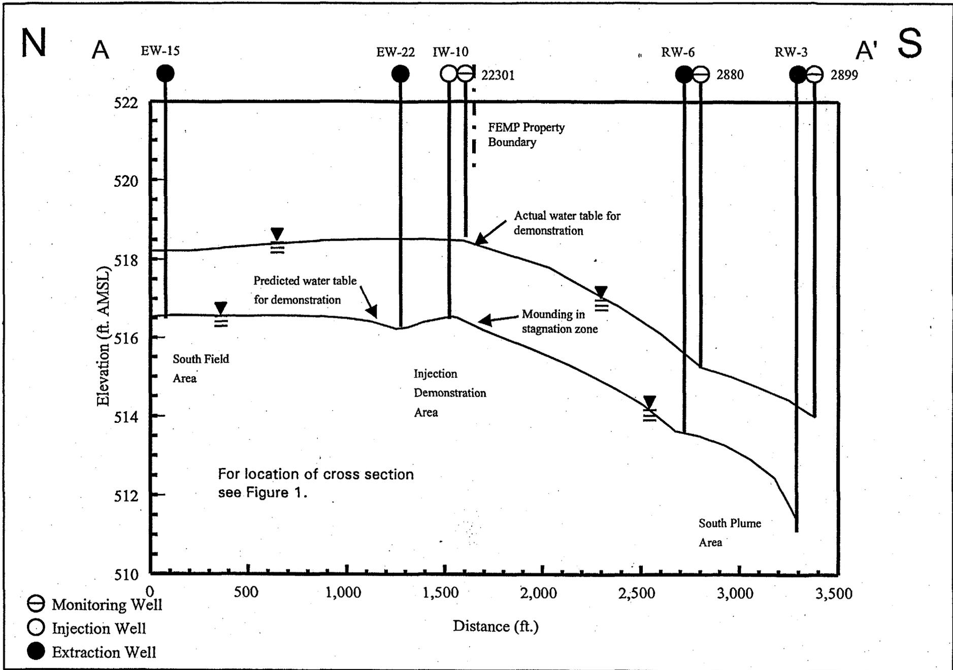
Figure 3. Measured Water Table Elevation Profile for Demonstration Time Period
