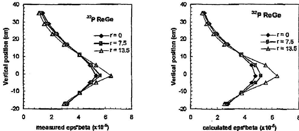
FIG. 1. Measured and calculated efficiency for high purity Ge detector and  $^{32}\text{P}$  isotope in the function of geometry relative to the detector plane and rotating radius of the waste drum.
