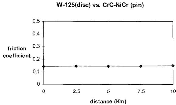
Fig. 4 Friction coefficient value in the first 10 km test
