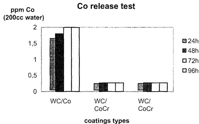
Fig. 2 Corrosion test in aqueous environment
