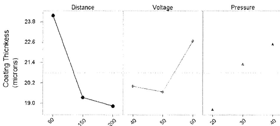
**Figure 4:** Optimization experiment main effect results from MINITAB software showing the effects of variation of substrate-electrode distance, spray gun voltage and air pressure on the ESC cBN coating thickness on carbide substrate. spray electrode voltage, and 3. air pressure. The values of control factor were varied to see the effect on ESC cBN coating, while keeping the other parameters constant.
