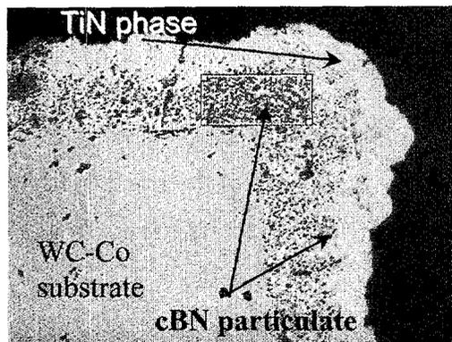
**Figure 6:** Cross-sectional view of ESC-CVI composite coating.
