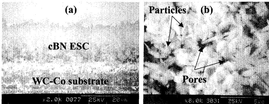
**Figure 3:** SEM micrographs, (a) cBN ESC layer on carbide substrate (2000x), and (b) ESC, cBN surface layer (8000x) showing cBN particles and porosity.
