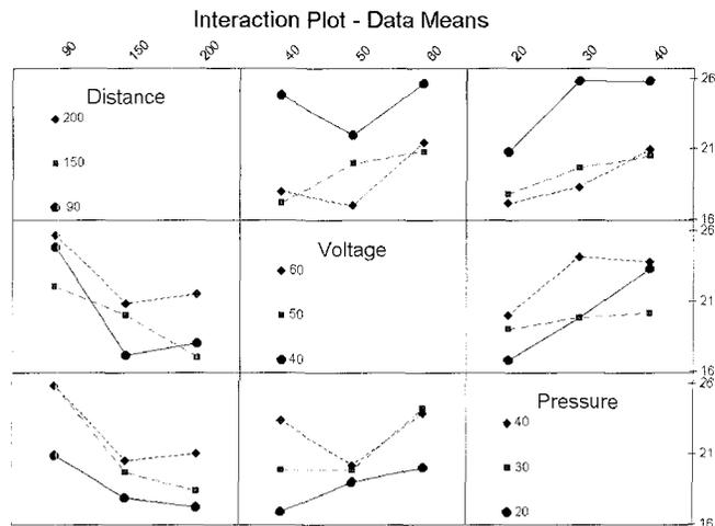
**Figure 5:** Optimization experiment interaction effect results from MINITAB software showing inter-parameter variation of control factors on the ESC cBN coating thickness on carbide substrate.
