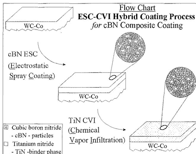
**Figure 1:** Schematic of the ESC-CVI hybrid technology.
