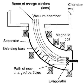
Figure 3. Schematic drawing of a separator devices
