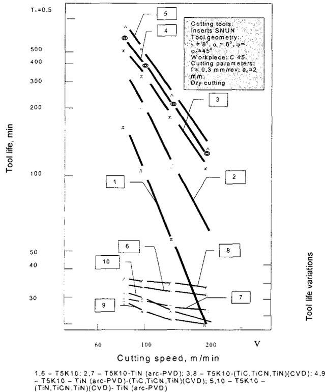
Figure 1. Tool life values of carbide with various combinations of coatings
