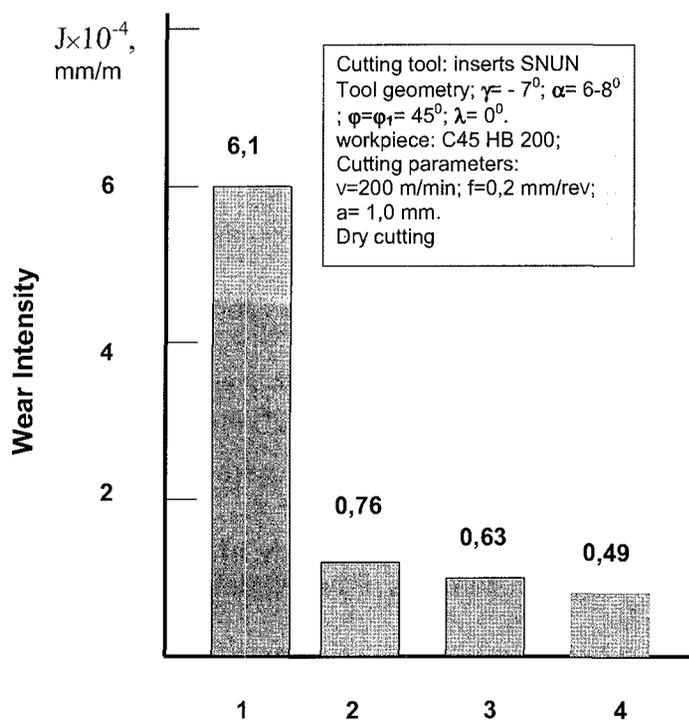
1 – control carbide; 2 – (TiC, TiCN, TiN) CVD; 3 – supermult. (TiCN) CVD; 4 – supermult. (TiCN) CVD - (TiAlN) - arc-PVD
