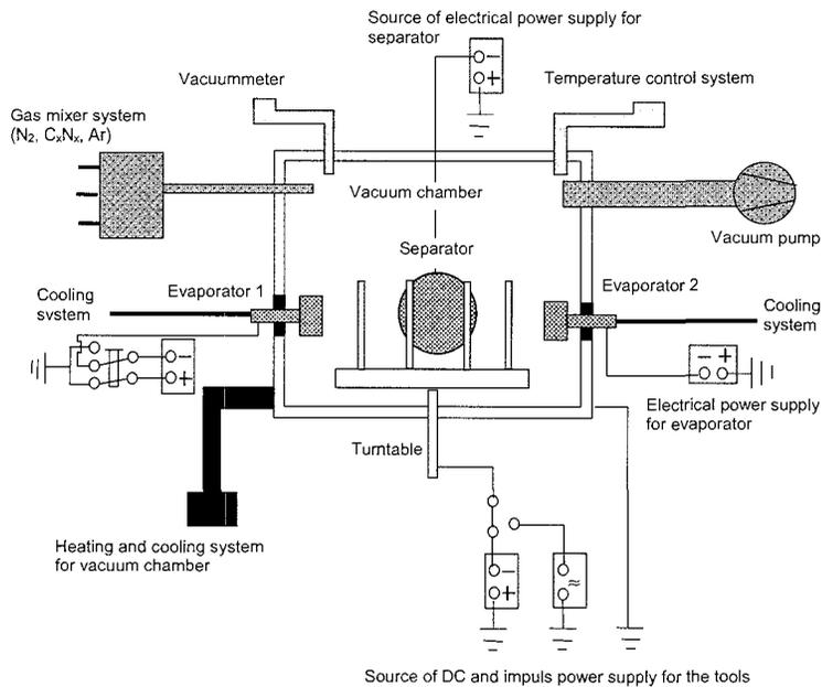
Figure 2. Schematic drawing of a vacuum-arc unit for combined ion plasma surface processing (CIPP) of cutting tools
