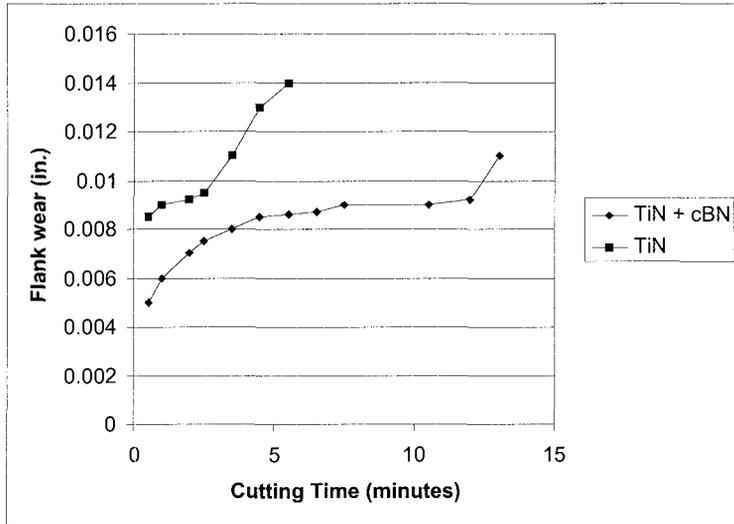
Fig. 4: Flank wear, Turning 4340 Steel, Rc 28-30 (600 sfm, 0.010 ipr, 0.08 in. DOC, CNGA432, dry machining)
