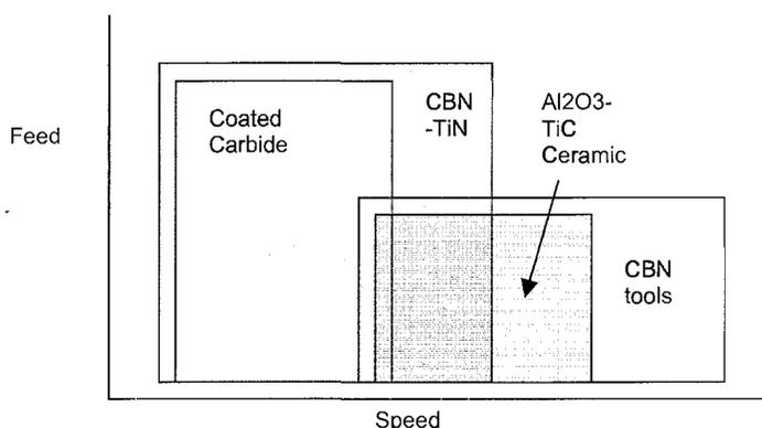
Fig. 8: Feed/speed diagram of anticipated performance range for composite cBN-TiN films on cemented carbide tools.
