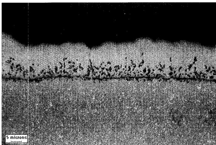
Fig. 3: Cross-section of TiN infiltrated cBN coating.
