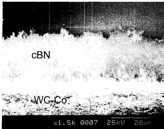
Fig. 2: SEM cross-section of ESC deposited cBN (1500X).
