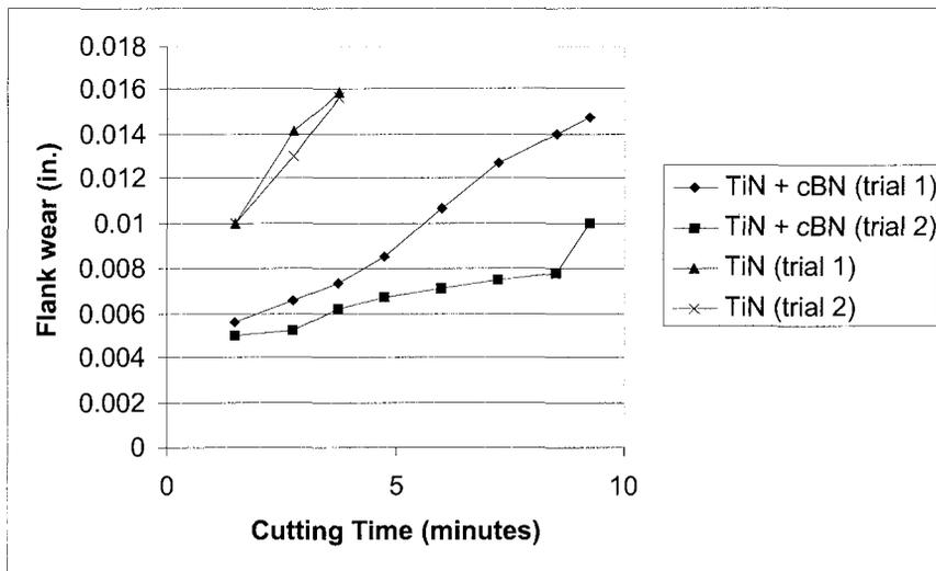
Fig. 5: Flank wear, Turning 4340 Steel, Rc 28-30 (600 sfm, 0.010 ipr, 0.08 in. DOC, CNGA432, dry machining)
