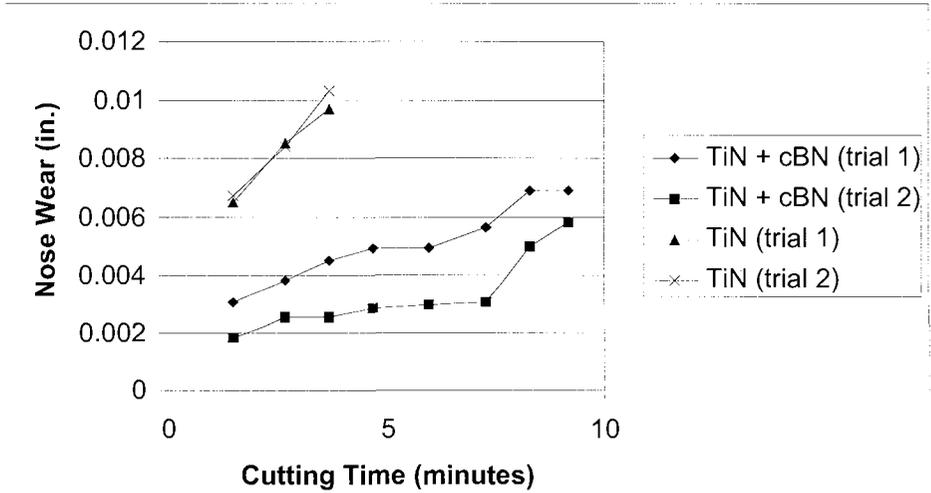
Fig. 6: Nose wear, Turning 4340 Steel, Rc 28-30 (600 sfm, 0.010 ipr, 0.08 in. DOC, CNGA432, dry machining)
